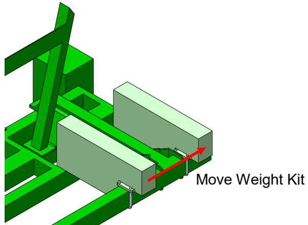
1. Using a 1/2" x 4 x 7-1/2" u-bolt, loosely attach 420-2820Y1 to rear 4x6 implement frame, outside of the 2x6 cross member.
