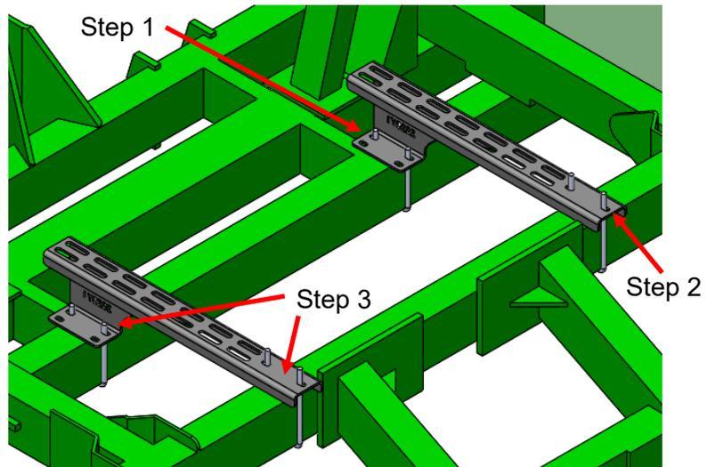
3. Place tank cradle/bracket on tank support brackets. Bolt loosely using 5/8" hex head bolts and 5/8" flange nuts.
