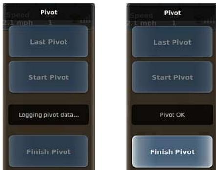
4. Press **Finish Pivot**. The panels close and the pivot path (with swath lines radiating outward) appears on the map.
