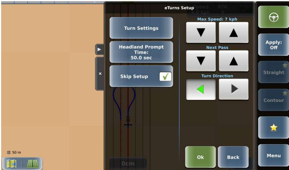
4. Press **Ok** to go to the eTurns Control panel, verify an acceptable speed (green speed bar at top of panel) and the correct turn direction, then press **Go**. The panels close and you begin guiding to the new actual eTurn path.
