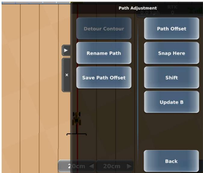
2. While still on the Path Adjustment panel, press **Save Path Offset**. The offset indicator disappears, the Save Path Offset button is disabled, and DISPLAY disengages.
