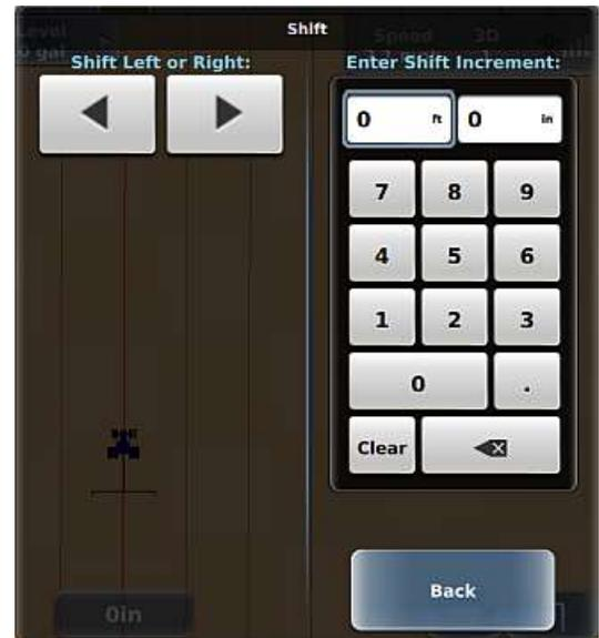
The guideline on the map moves by the selected direction and shift amount and a shift indicator appears (see below) to the left or right (based on the shift direction) of the crosstrack indicator (figure below shows a shift left of 3 feet).
