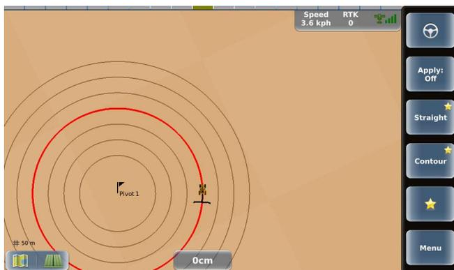
5. Press the engage button to engage automated steering. DISPLAY steers your vehicle along the pivot guideline.
