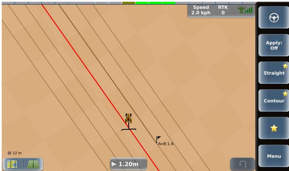
5. Press the engage button to engage automated steering. DISPLAY steers your vehicle along the A + Direction line.
