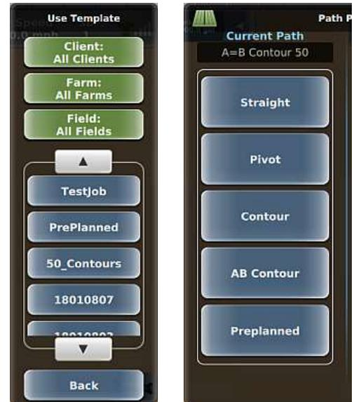
4. Press **Preplanned**. The panel closes and the template appears on the map. The example below shows a boundary (blue), guidelines (gray/brown), and nearest guideline (red). When a guideline is red you can engage on that line using autosteering (provided all engage conditions are met).
