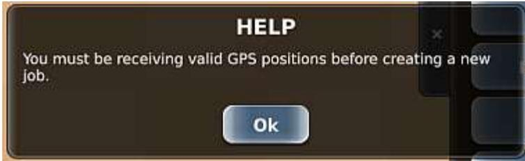
This message appears when attempt to create a new job (New Job button on the Jobs panel is disabled) with no GPS. Close the message, examine your system and take the necessary steps to obtain a GPS signal (such as verifying no cables are loose), then try again to create a new job.
