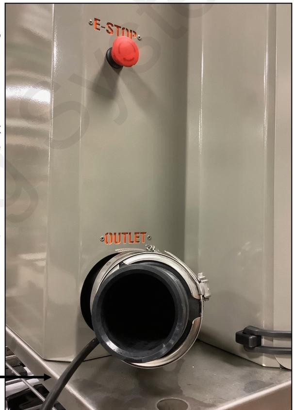
Be sure the outlet of the drain tube is in a place where it is safe to discharge the liquid that will be drained.
