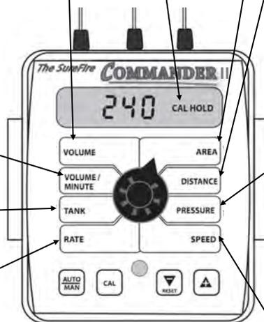
**CONTROL SPEED:** Default for Anhydrous is -1. Adjust as needed for stable operation in the field.
