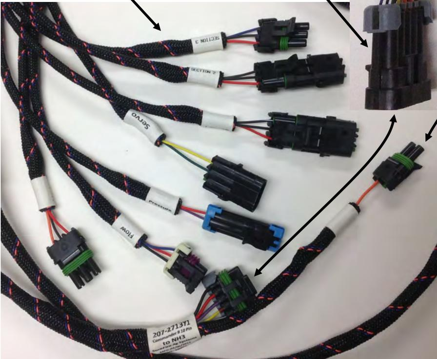
EMD ENABLE on 18034 plugs into MASTER 2-pin on 207-2713Y1
