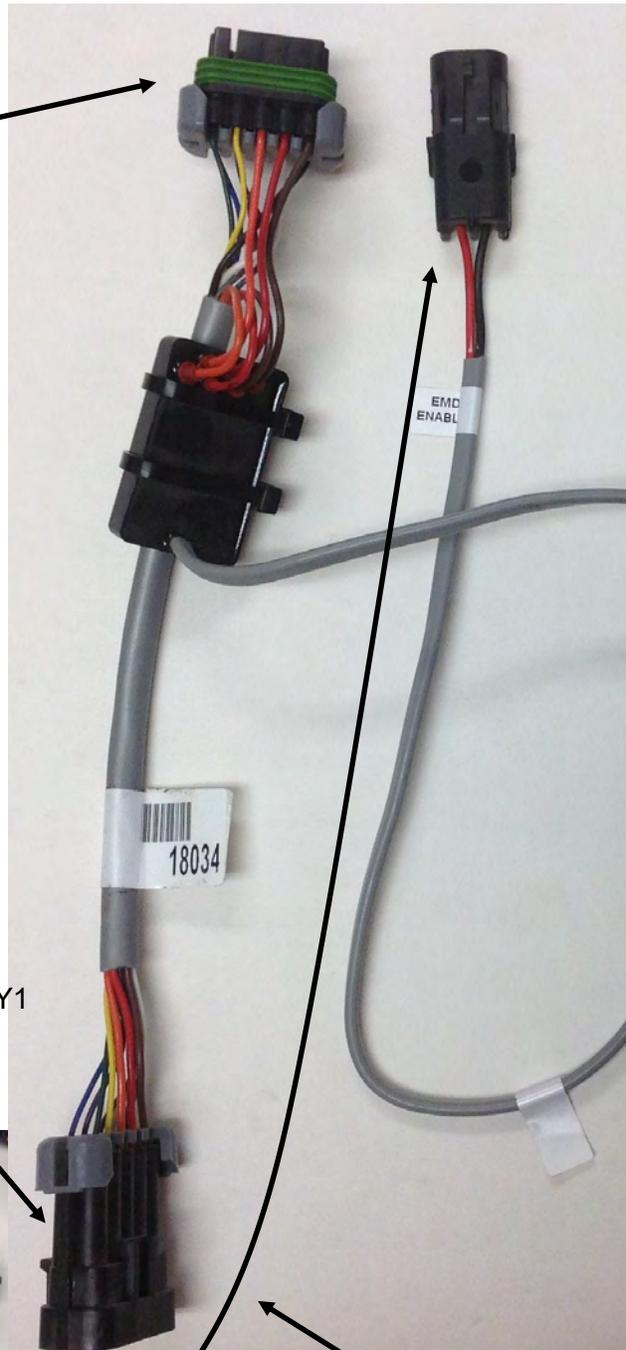
Connectors on 207-2713Y1 for Flowmeter, Master ON/OFF valve, servo control valve, pressure, Section 1, Section 2, Section 3.
