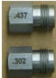
**Correct orifice must be installed before use.**
