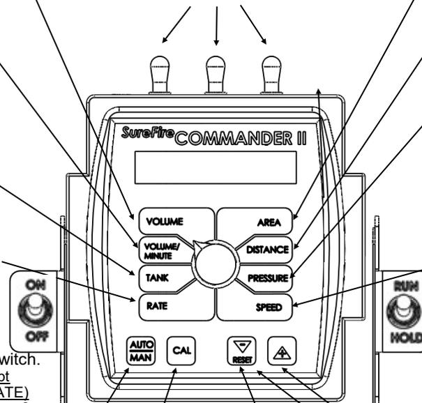
**RUN/HOLD:** Turns anhydrous application on (RUN) or off (HOLD)
