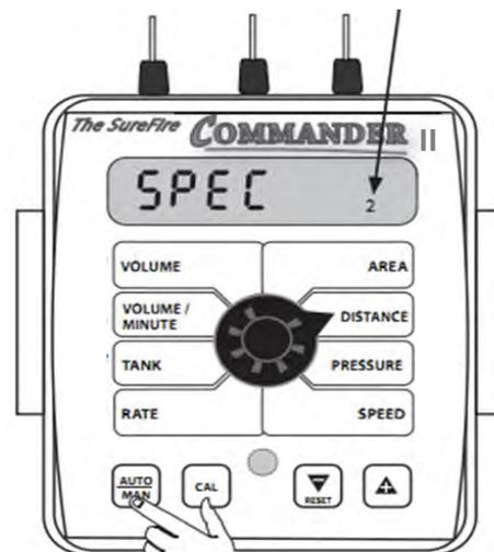
**NOTE: The above procedure will load all default values in the Commander II. It must be done before standard calibration.** For example, if you entered your implement width, then did the quick setup above, the Commander II would default back to 240 inches.
