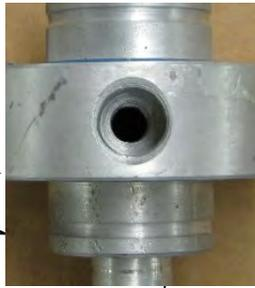
Threaded orifice not installed
