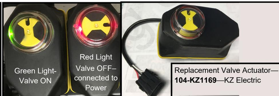
**This is a 3-way valve.** If product will not flow when valve is ON, either move the outlet hose to the other port, or remove actuator and rotate valve ball 180°, and replace actuator. . Product should flow through the port closest to the Indicator light when the valve is open (green).
