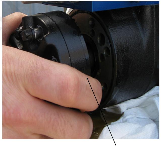
Pull these three sections away from the motor body to jump the "dog bone" shaft 1 tooth. This will reverse the motor rotation.
