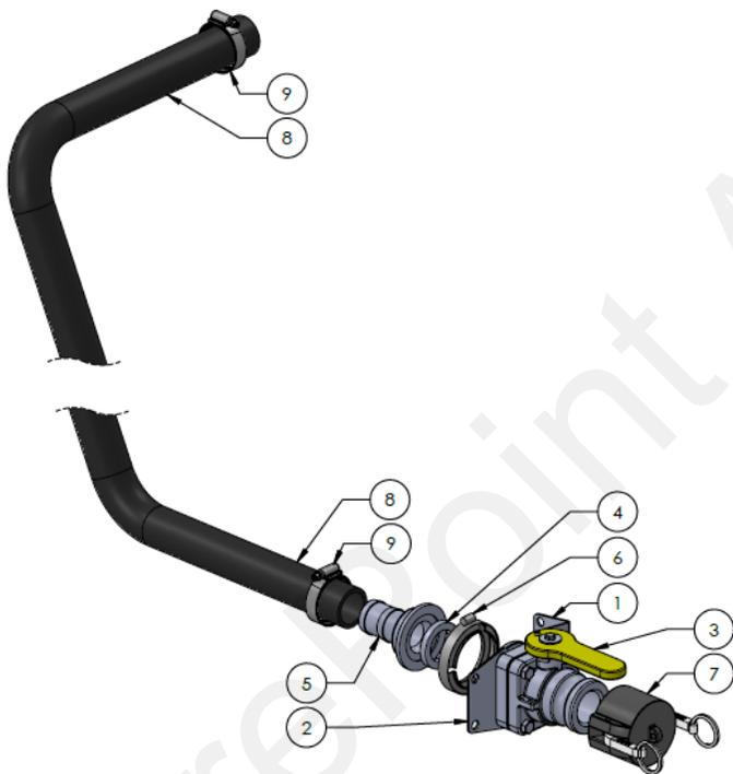
1. Assemble fittings as shown below, using manifold clamp and gaskets.
