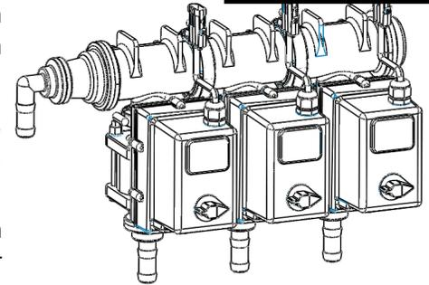
3. Check voltage pin A to Pin B. Must be 12 volts, if not, go back to 10-pin on Commander II and check voltage (pins J & K, white and black wire).
