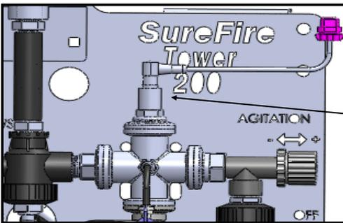
The pressure transducer is factory calibrated and will display a very accurate pressure reading on the Commander II. No manual gauge is required.
