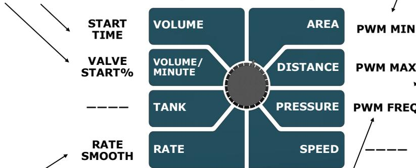
**PWM MIN %:** This setting affects how low the PWM signal can go. If set to 10, then the PWM signal can go down to 10%. If set to 20, then the PWM signal can go down to 20%. Most valves have a bottom end where they no longer change any flow. This is the point where the PWM MIN should be set. If this is set too high, it will keep the system from getting to your lowest rates.
