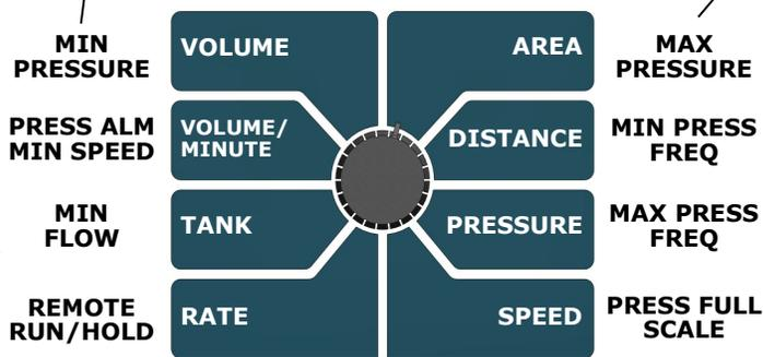
**MAX PRESSURE:** The system alarms if the pressure gets above this setting. This cannot be set higher than the pressure full scale setting.
