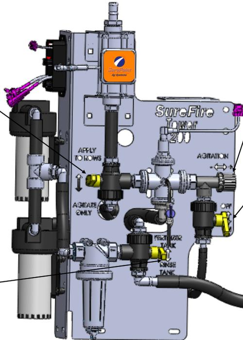
**Agitation Adjust Valve:** This valve adjusts how much flow returns to the tank while working in the field. *(If using, start with a 1/4 to 1/2 turn.)*
