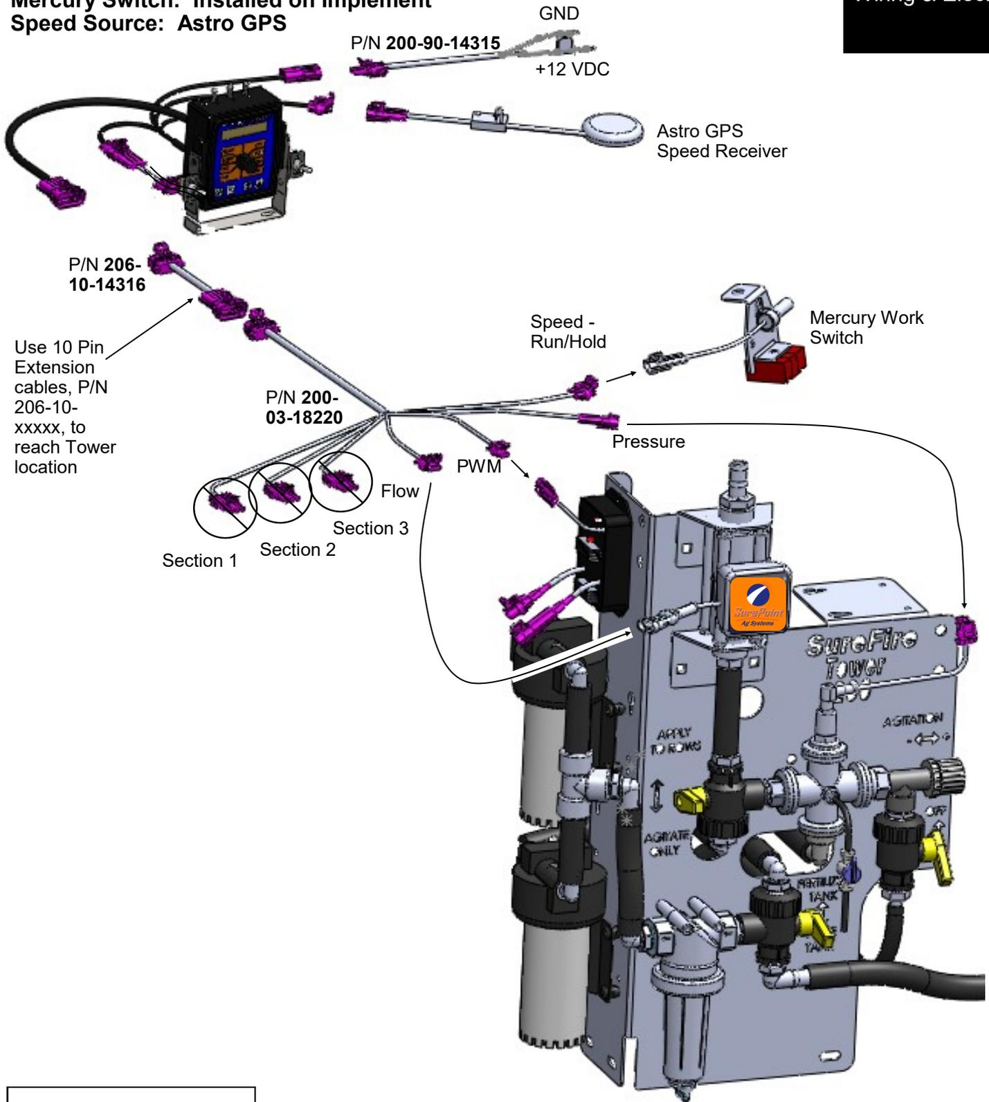
Use 10 Pin Extension cables, P/N 206-10-xxxx, to reach Tower location
