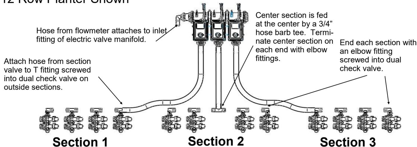
Hose from flowmeter attaches to inlet fitting of electric valve manifold.
