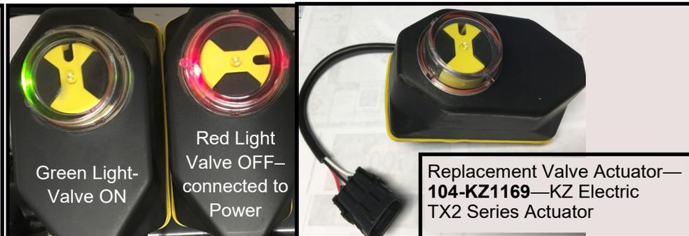
**This is a 3-way valve.** If product will not flow when valve is ON, either move the outlet hose to the other outlet port, or remove actuator and rotate valve ball 180°, and replace actuator. Product should flow through the port closest to the Indicator light when the valve is open (green).
