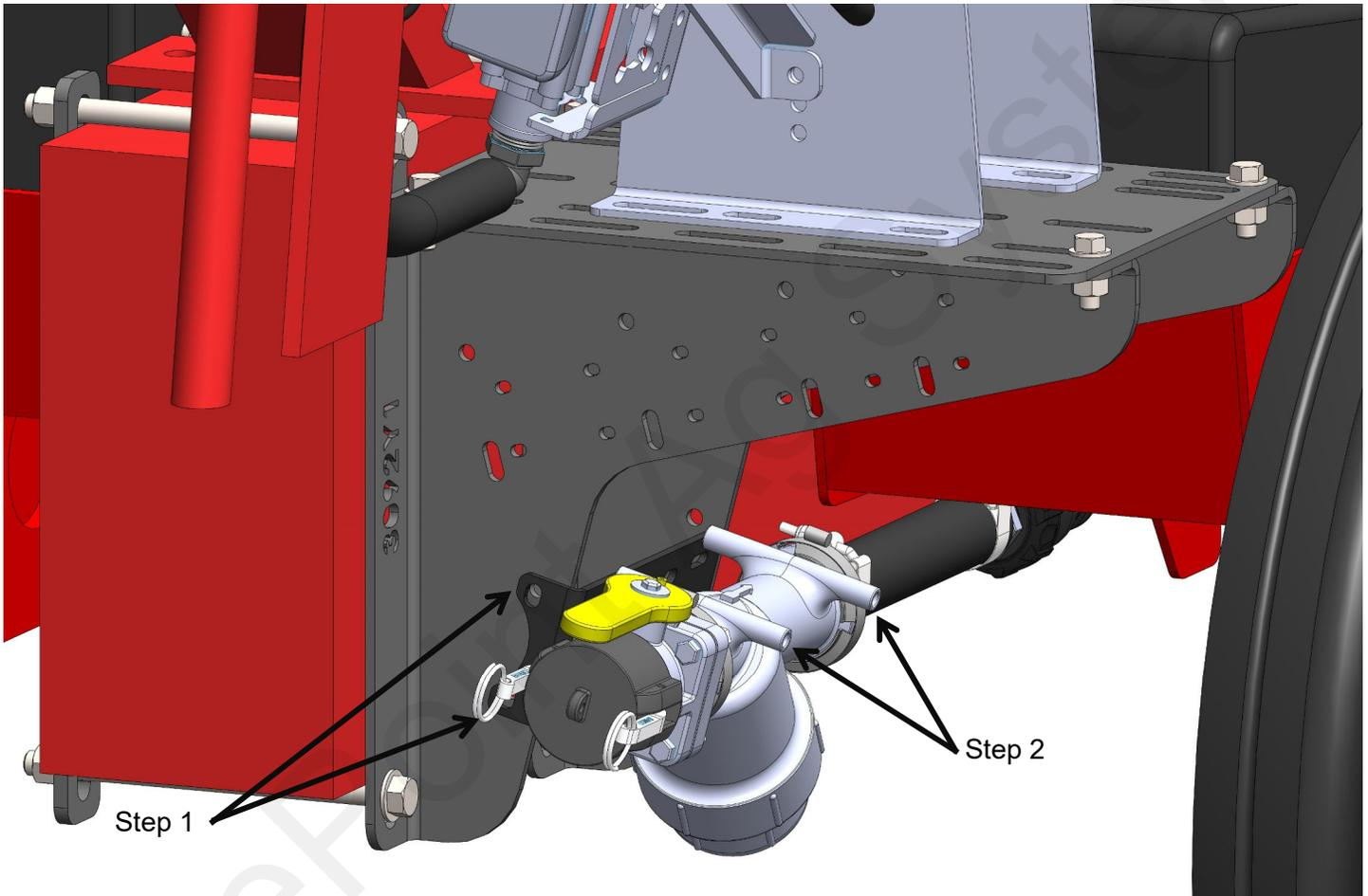
1. Mount universal fill kit bracket, part number 400-2605Y1 (sold separately), to the front or rear pump mounting bracket holes using two (2) 3/8" x 3/4" hex head bolts and flange nuts as shown.
