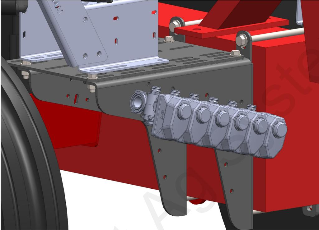
Up to three (3) Banjo Section Valves may be u-bolted to the side of the pump support bracket using the larger bolt hole and slotted hole in the center as illustrated below.
