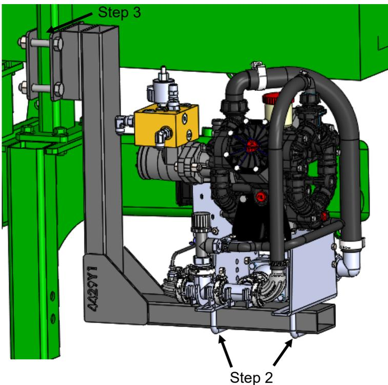
2. Mount PumpRight Pump on Horizontal bar of 410-4429Y1 Bracket using the supplied 1/2" U-bolts. Pump can be mounted 180 degrees from what picture on left shows per your preference on pump inlet and outlet locations.
