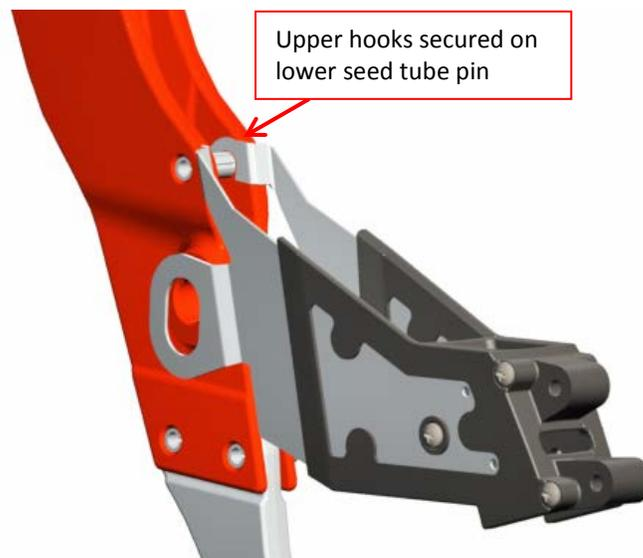
Illustration 3 – Quick Attach Firmer Bracket Installed
