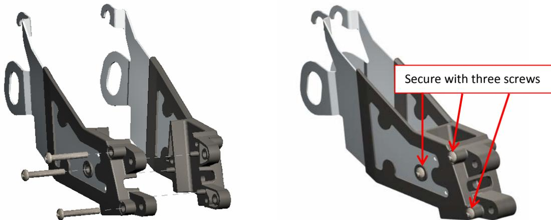
Illustration 2 – Assemble Quick Attach Firmer Bracket
