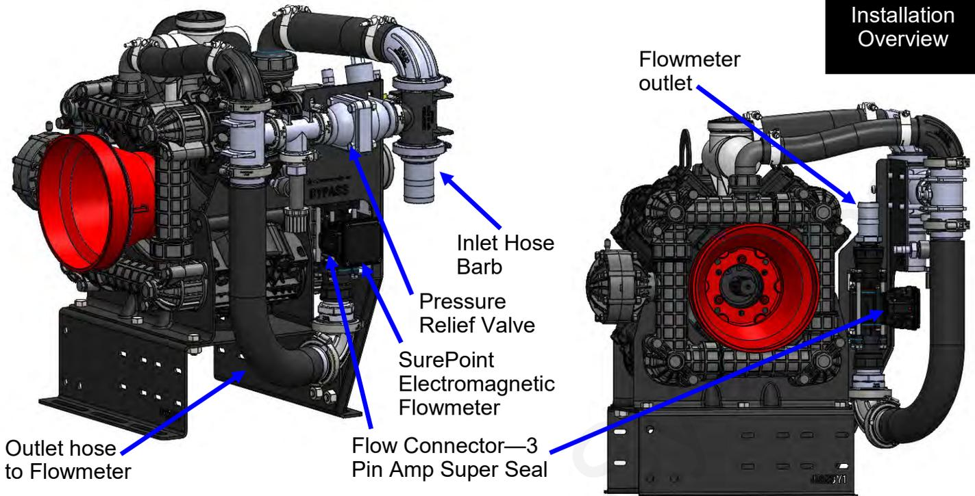
**Inlet:** The PR80 PumpRight is shipped with a 2" inlet hose barb. Attach this to the hose from your supply tank and strainer. A 2" 90 degree hose barb is included and can be substituted. In high flow scenarios, use a 3" inlet hose and replace the 2" hose barb with a 3" reducer coupling.
