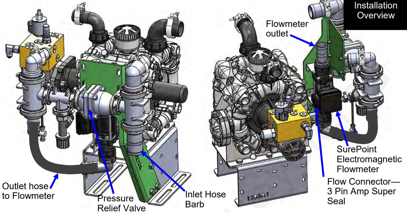
**Inlet:** The PR40 and D250 PumpRight are shipped with a 2" inlet hose barb. Attach this to the hose from your supply tank and strainer. A 2" 90 degree hose barb is included and can be substituted.
