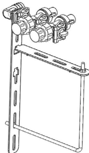
**Example 3.** Use the long bracket on the front of a 3x7 bar (vacuum tube on some planters). Mount the check valve hanging forward of the bar.
