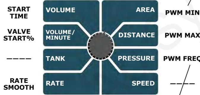
**PWM MIN %:** This setting affects how low the PWM signal can go. If set to 10, then the PWM signal can go down to 10%. If set to 20, then the PWM signal can go down to 20%. Most valves have a bottom end where they no longer change any flow. This is the point where the PWM MIN should be set. If this is set too high, it will keep the system from getting to your lowest rates.
