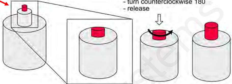
**Manual Override** - Override will completely open valve, so turn down the hydraulic flow in the cab.
