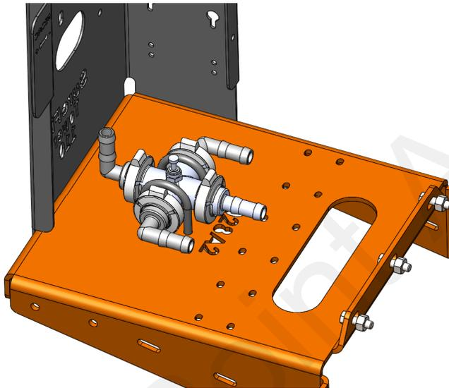
2. If section valves are not used, mount BOM 520-00-045000 (instruction sheet 396-2602Y1) as shown at left.
