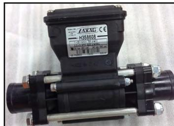
Serial number label on side also shows pulses per gallon.
