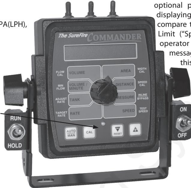
**SPEED:** Displays ground speed in miles per hour (kilometers per hour).
