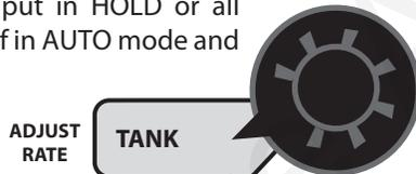
**AUTO DELAY TIME:** Typically used when using relatively slow ball valves for boom shut-off, this feature delays adjustment of the servo valve until the boom valves are open. Use “+” and “-” buttons to set from zero (OFF) to 4 seconds.
