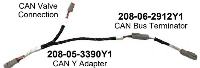
3. **2nd Option:** If CAN Valves are not in close proximity, use the appropriate length extension harness to route from the **Bus Extension/Termination** connector in the QuickDraw to the closest CAN Valve. Use CAN Y Adapter (208-05-3390Y1) to connect to the valve and extension cable to the next valve. Repeat until all valves are connected, re-use CAN bus terminator harness (208-06-2912Y1) at the final Y adapter.
