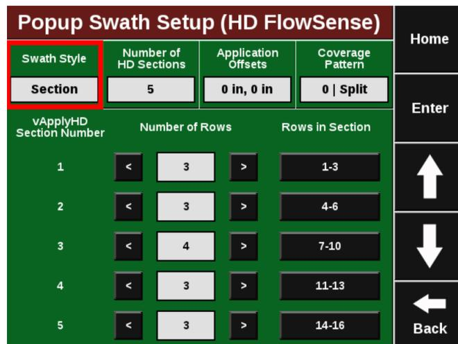
**Section:** This option allows the operator to customize the swath sections. Set the total number of swath sections at the top of the screen. Then use the arrows to assign rows to sections or press on the “Rows in Section” box to list rows in the section.
