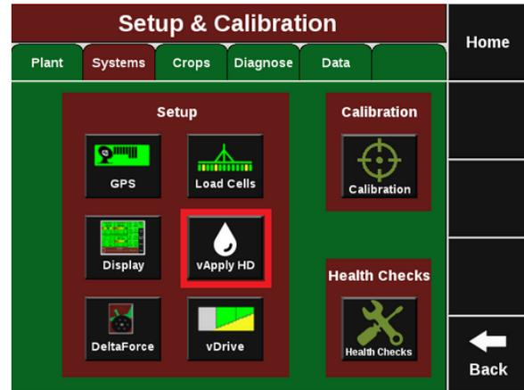
For single vApplyHD systems only, the first product setup will need to be completed. Press on the Product 1 setup button on the top left side to begin the setup process. For multiple liquid systems (vApplyHD and/or FlowSense) each system will need to be setup individually. Up to four liquid systems can be configured.
