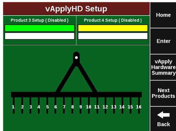
To successfully configure a vApplyHD system all settings on this page must be set correctly. In order for the liquid product to be viewed on the home page and diagnose page the Control Style and Product Nickname must be set.
