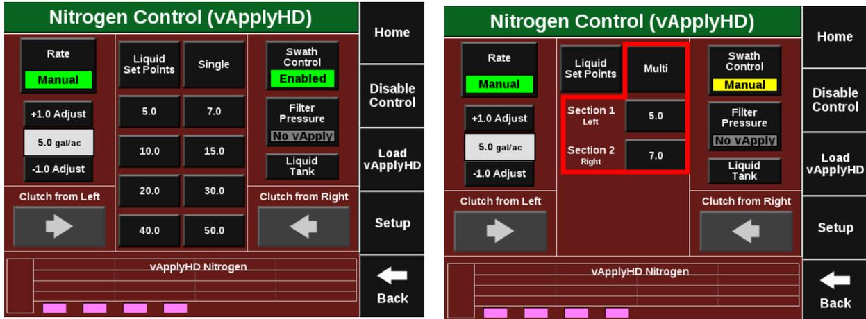
Within manual mode the operator can choose a single rate or multiple manual rates. To change between “Single” and “Multi”, select the button at the top center of the screen. If “Single” is showing, the planter will apply a single rate across all rows. If “Multi” is showing, a different rate can be assigned to each drive section. (Drive sections must be configured in the vDrive setup.) Change the rate for each drive section by pressing on the rate displayed next to each section number.
