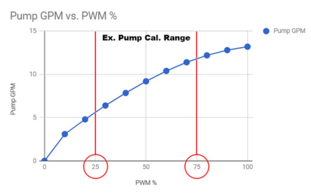
A successful Pump Calibration will set a Min and Max PWM percentage based on the total pump GPM achievable at those commands. This is the operation window that vApply expects to run within but does NOT keep vApply from operating outside of this window. In the event that the current speed and rate combination is outside of this window, vApply will use the pump curve to command the needed PWM.
