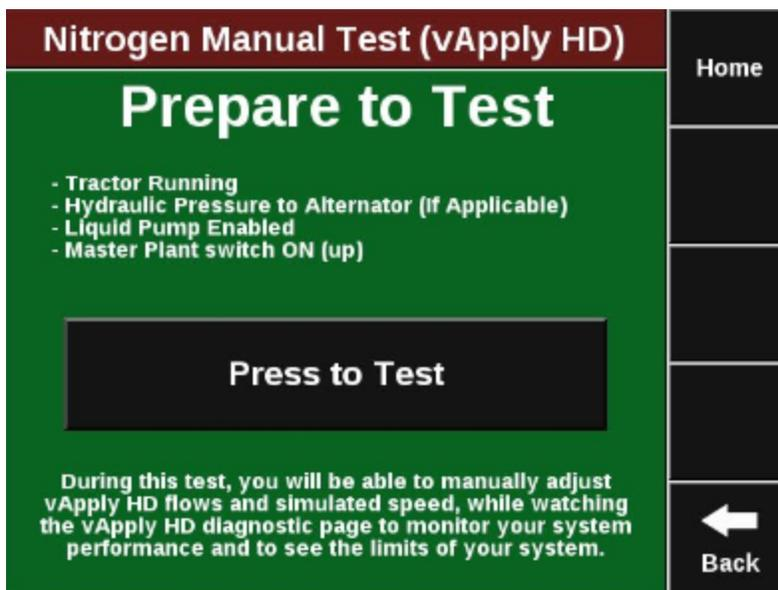
Select “Press to Test” to begin the test. This test will allow the user to enter simulated speed and product rates they may encounter when using vApplyHD. Use this mode to check for plumbing leaks after initial vApplyHD installation.
