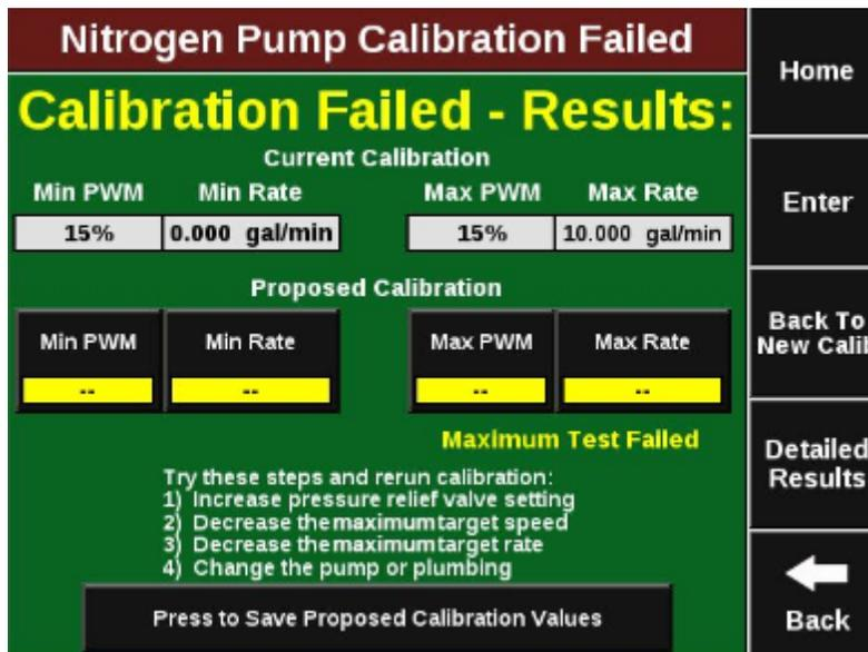
This Calibration process will typically fail the first time and requires adjustments to be made to the system prior to a successful calibration. Three or more attempts may be necessary to set up a vApplyHD system.
