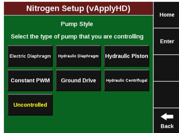
**Note:** The vApply Module will only control electric or hydraulic pumps that are equipped with a PWM driver or valve.
