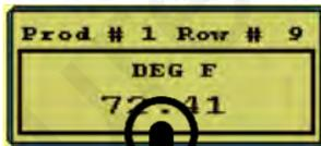
From the HOME screen, touching the row detail button will display the row detail page. The user can toggle through the rows by touching the < > buttons. The user can also pause the **Auto Scrolling** feature pressing the **Pause Scan** button.
