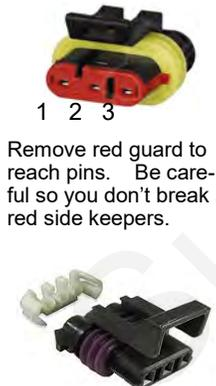
Remove red guard to reach pins. Be careful so you don't break red side keepers.
