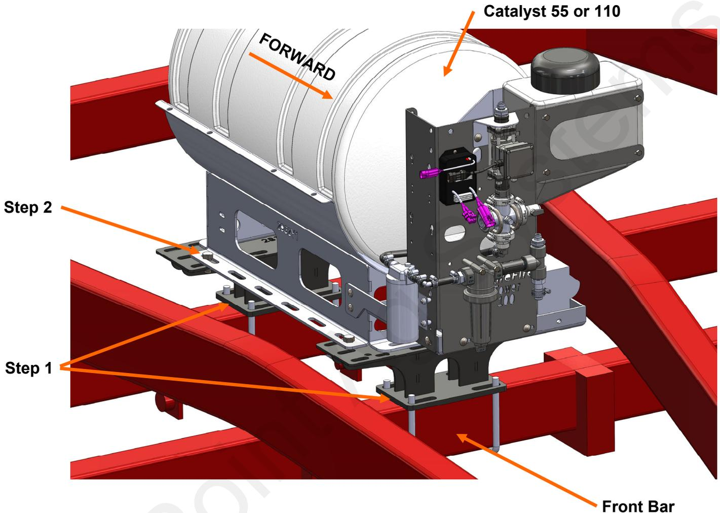
1. Center mount the two provided 420-2815Y1 Pedestals with provided 380-1041 Square Bend U-bolts as shown in picture above. Do not tighten U-bolts for adjustment in next step.
