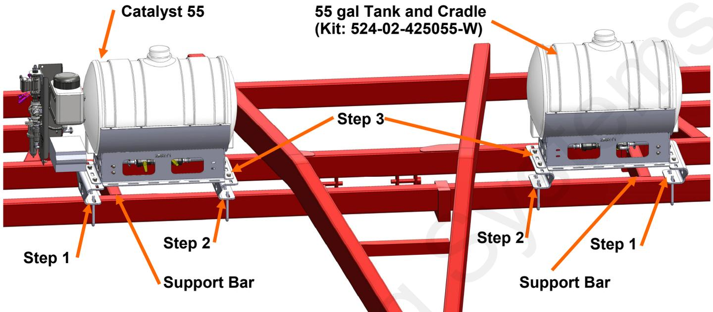
1. Mount the two outside 420-2986Y1 Pedestals with the provided 380-1041 Square Bend U-bolts first. They should go on the outside edge of the support bars on each side of the Implement as shown in Picture above. Do not tighten to allow for adjustment in next steps.
