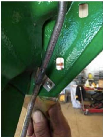
3. Slide ExactEmerge Fertilizer tube over disc bolt as shown. This bracket takes the place of two (2) shims. It is the exact width of two (2) shims.
