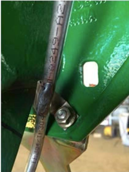
6. Align the tube so it is in the center of the seed tube guard and pinch the tab tightly around the guard with a channel lock. (We find a channel lock works the best.)
