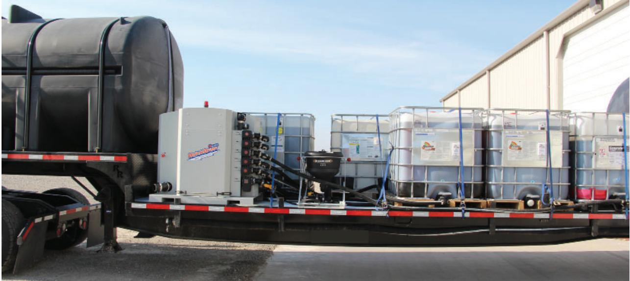
**QuickDraw on drop-deck trailer. Water tanks front and back. Locations for 7 chemical totes. QD swing-down eductor for ground level working.**
