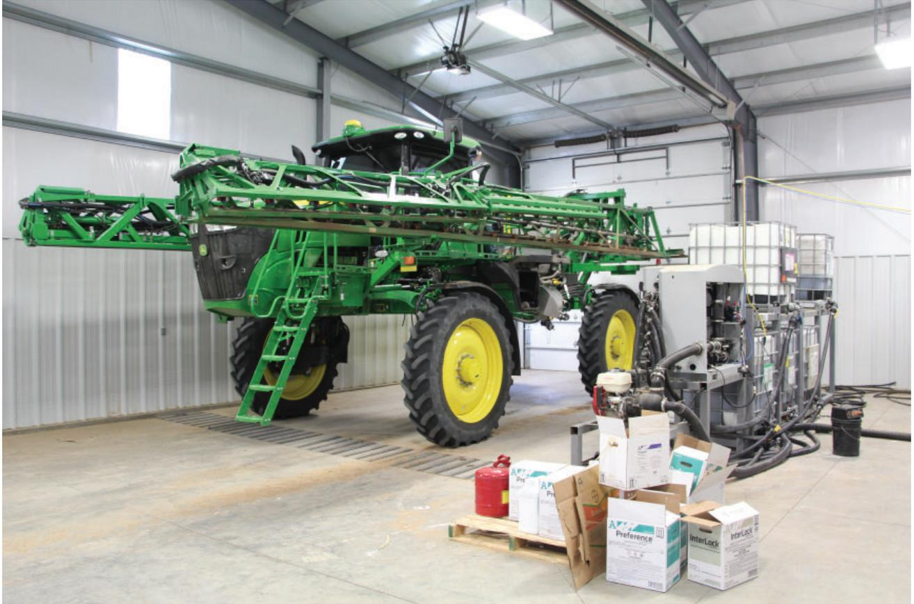
**Farmer with dedicated “spray shed”. Either load directly into sprayer or mix “hot load” to be hauled to the sprayer.**
