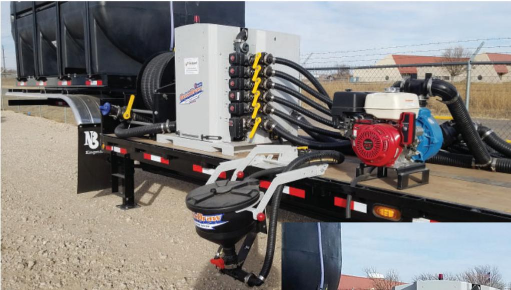
**QuickDraw on drop-deck. Front and rear water storage. Electric 3" hose reel and locations for 6 chemical totes.**
