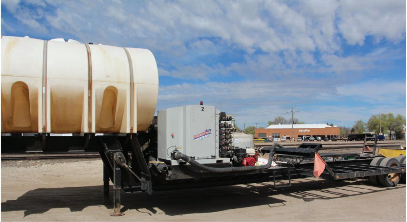
**QuickDraw installed on sprayer transport trailer.**
