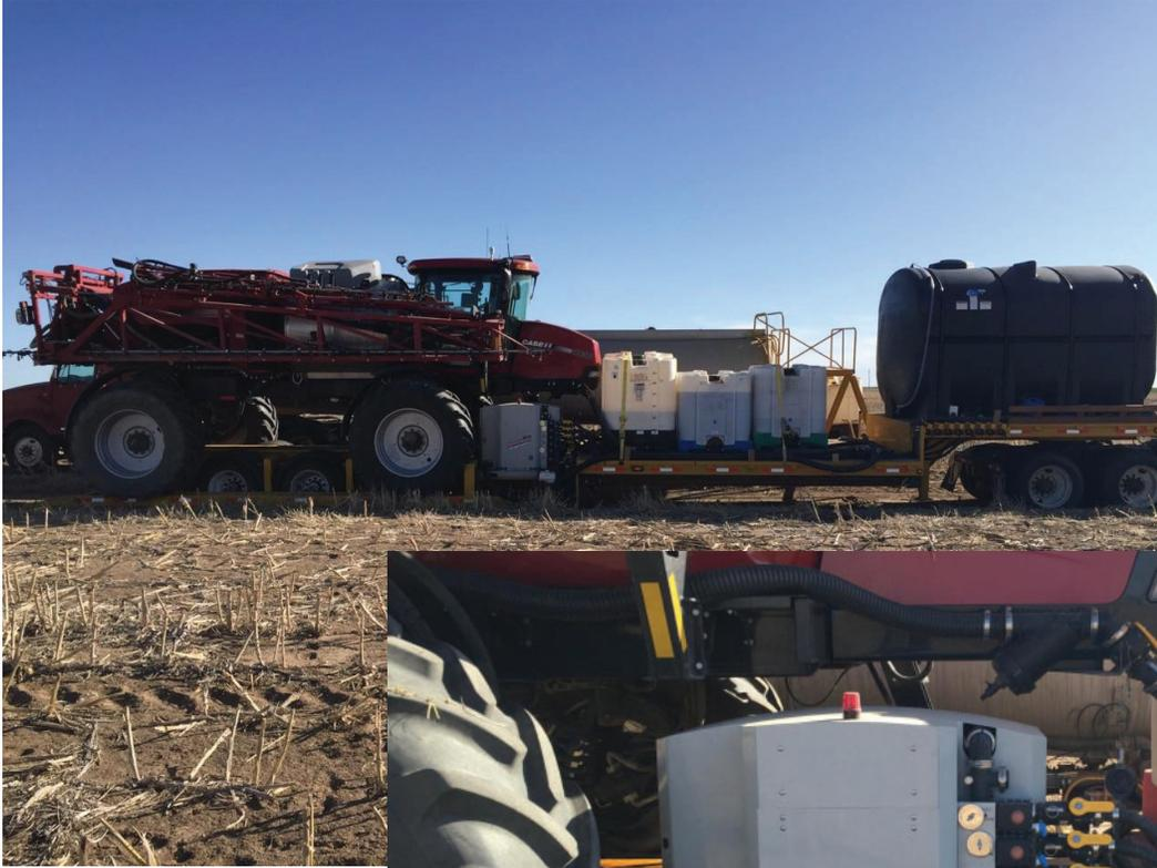
**QuickDraw installed on sprayer transport trailer.**
