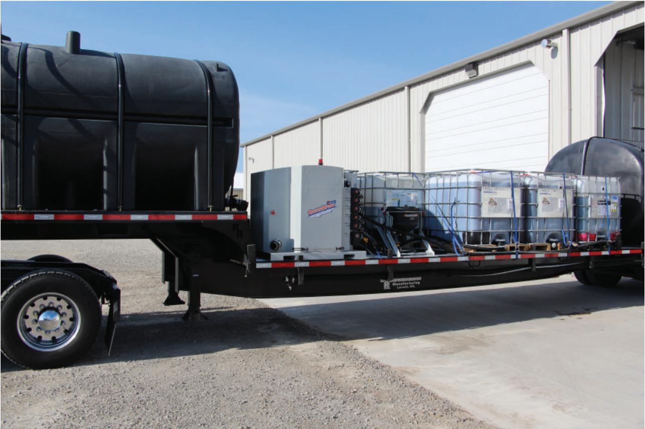
**QuickDraw on drop-deck trailer. Water tanks front and back. Locations for 7 chemical totes. QD swing-down eductor for ground level working.**
