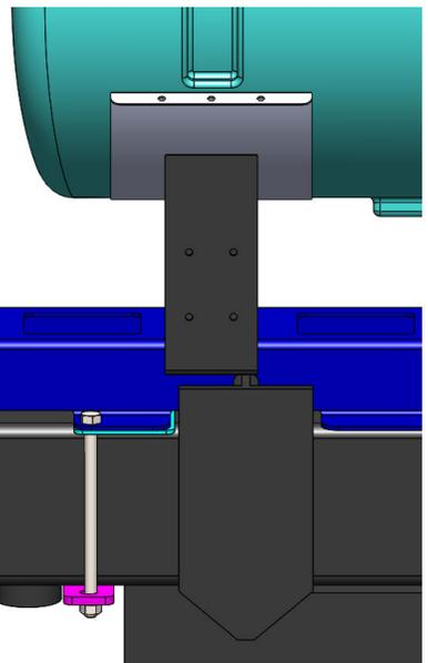
7. Bolt tower mounting bracket to attachment bracket in front of tank using four 1/2" bolts, washers, and flange nuts. Tower will bolt to this bracket with 3/8" carriage bolts.
