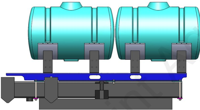
4. Loosely bolt tank saddles to attachment bracket using 1/2" bolts, washers, and flange nuts.
