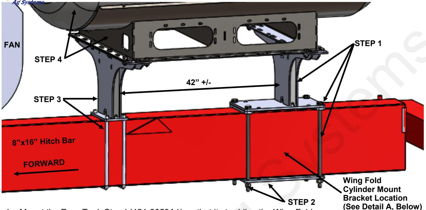
1. Mount the Rear Tank Stand (421-2059A1) so that it straddles the Wing Fold Cylinder Mount Bracket (See Detail A, Below) attached to the 8"x16" Hitch Bar towards the rear. Place the Spacer Brackets (421-2274Y1) underneath the Rear Tank Stand as shown in picture above. Insert 3/4"x20" Long Bolts with Washers through Rear Tank Stand and Spacer Brackets.
