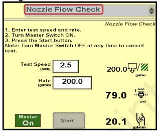
Use **Nozzle Flow Check** to see if system will lock on to a **Rate** at a **Test Tpeed**. You can change speed or rate while the test is running.
