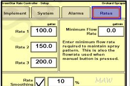
Control Valve Calibration: If the system will not lock on to Rate when applying, change from 2512 to 2533. If the Rate is still unstable, go to 2033. If still unstable, go to 1533.
