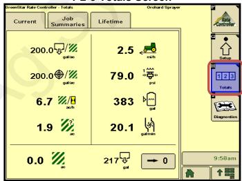
**Diagnostics—Readings—Delivery System** will show details on *flowmeter* operation, *flow (gal/min)*, and *spray rate (gal/ac)*. This can be useful information for troubleshooting.
