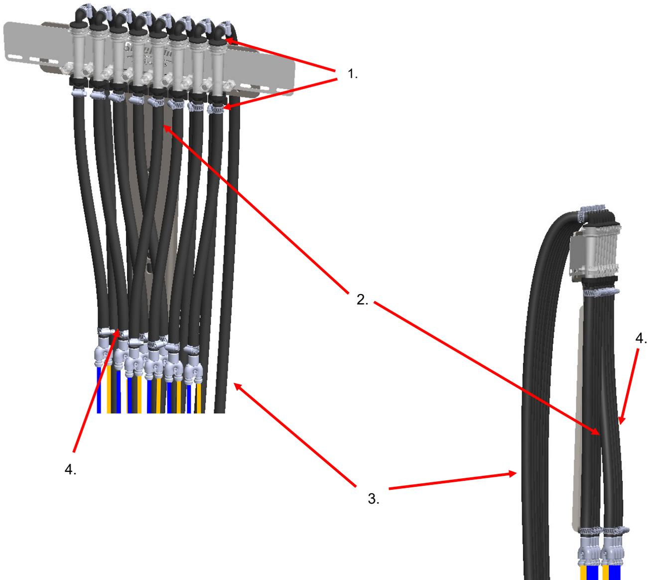
*Gen3 LiquiShift installation is the cleanest when Flow Indicators / Sentinel Flowmeter Modules are distributed across the toolbar.*
