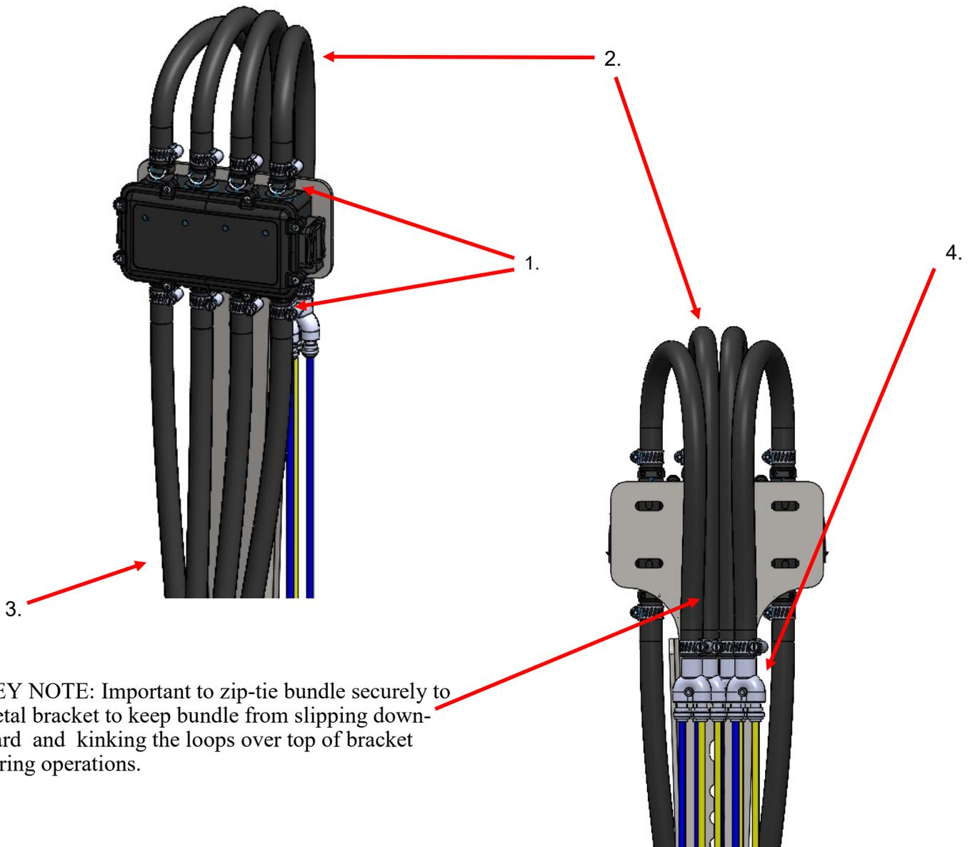
**KEY NOTE:** Important to zip-tie bundle securely to metal bracket to keep bundle from slipping downward and kinking the loops over top of bracket during operations.
