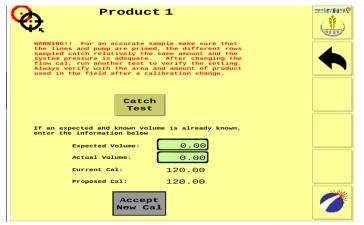
While the test is running, the actual rate and Flow per Minute will be shown. The Volume Target is the volume per row multiplied by the number of rows being caught. When the Volume Target for the test rows is reached, the test will stop. Add together the amount caught in all the rows tested. Enter this amount in **Actual Volume.**
