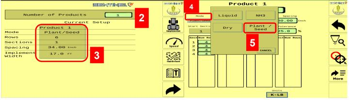
If you are running multiple drive motors you will have multiple PWM sections. With multiple PWM sections you will have to set a calibration number for each individually driven section. The best way to do this is to do a catch test for one section, then set that as the calibration for all of the sections. Next you will need to do catch tests for **each** section to verify you have the correct calibration number for each section.
