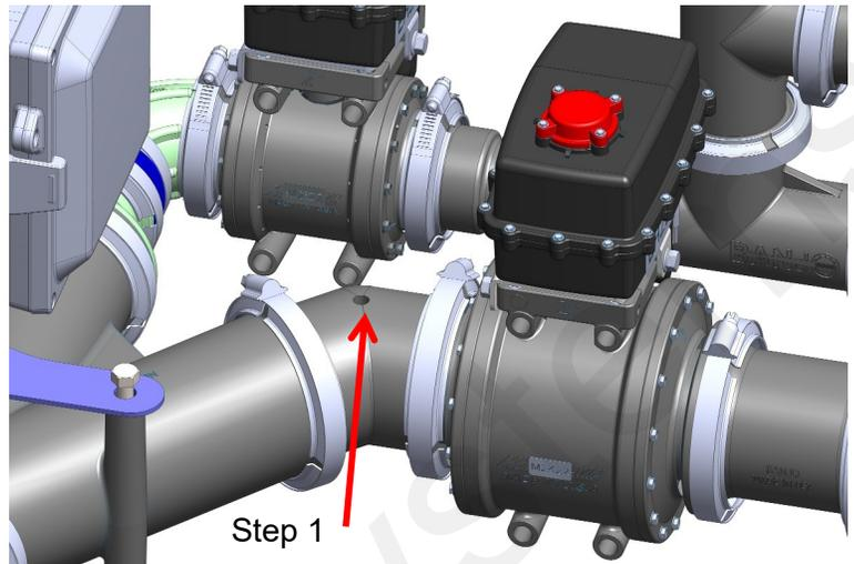
2. Insert tapped 2" manifold coupling (Item 9) with clamp and gasket (Items 7 & 8) between check valve and hose barb fitting with tapped 3/8" hole facing the general direction of 45° coupling.
