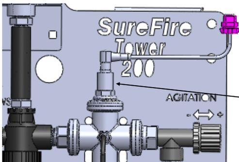
Pressure Sensor (3-wire type) with harness
