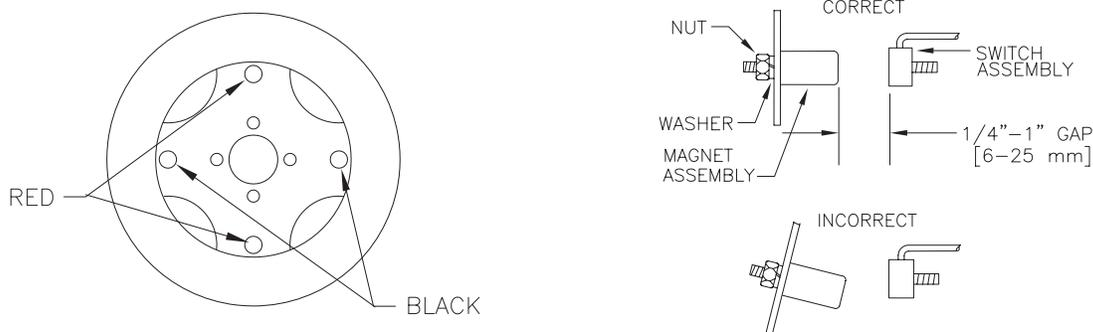
2. Mount the four magnets in the pre-punched or drilled mounting holes on the inside of the wheel so that the red magnets are on opposite sides of the wheel.
