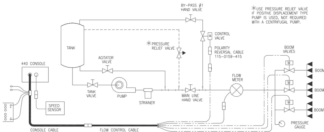
**Note:** This plumbing schematic applies only to applications of less than 3 GPM [11 lit/min]. For flow of 3 GPM [11 lit/min] or greater, the motorized control valve is installed on the main hose line. Refer to the Install the Control Valve section on page 18 for the main hose line plumbing procedure.
