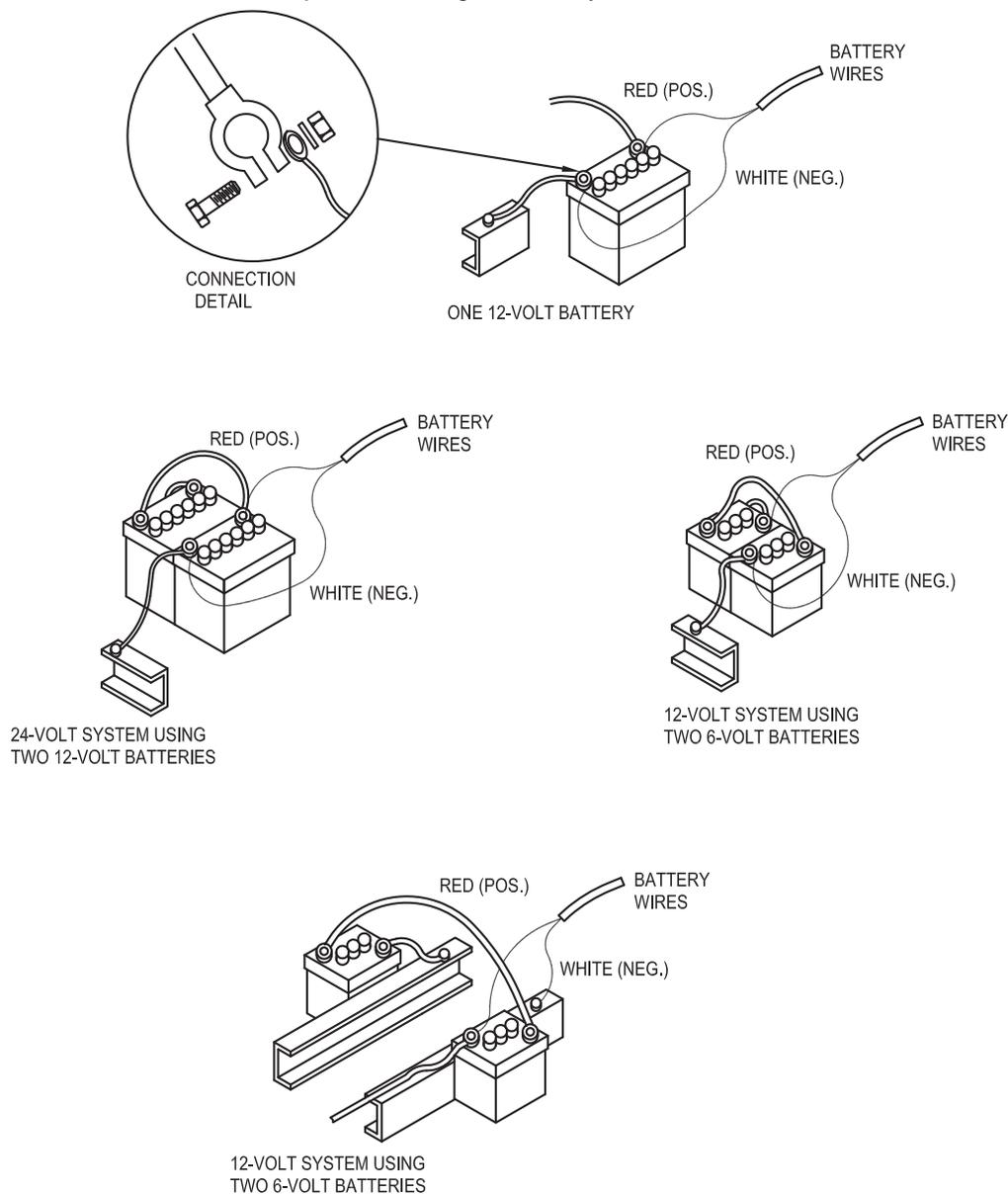
1. Route the red wire on the console control cable to the 12 VDC battery and connect it to the positive (+) battery terminal.
