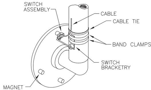
**Note:** The switch assembly does not need to pivot with the wheel.
