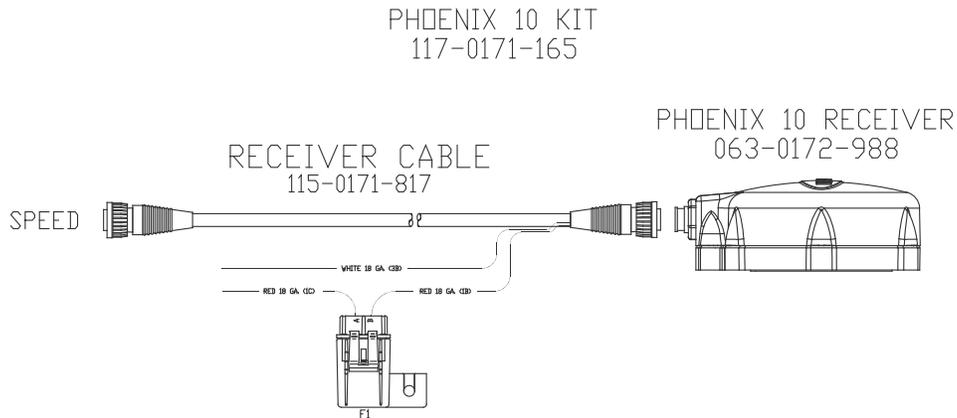
**Note:** The Phoenix 10 is powered by a 9 - 16 VDC negative ground system.
