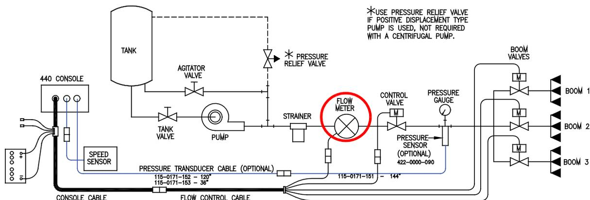
**Note:** All flow through the flow meter must go to the boom sections only. Ensure there are no return, agitation, or sparge lines to the tank or pump after the flow meter.
