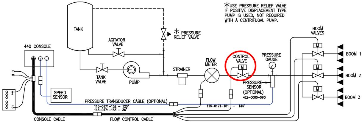
**Note:** This plumbing schematic applies only to applications of 3 GPM [11 lit/min] or greater. For flow less than 3 GPM [11 lit/min], the motorized control valve is mounted on a bypass line. Refer to the Alternate Bypass Line Plumbing System section on page 19 for the alternate bypass line plumbing procedure.
