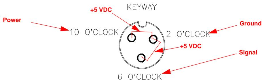
**Note:** If a +5 VDC voltage reading is not present, disconnect the speed sensor cable. If the flow reading is restored, refer to the *Testing Speed Sensor Extension Cables* section on page 46 to test the speed sensor extension cables.
