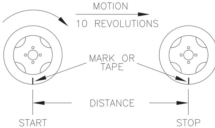
1. Place a chalk mark or tape on the tire on which the speed sensor is mounted.
