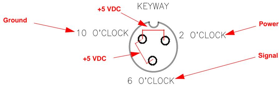
**Note:** If a +5 VDC voltage reading is not present, disconnect the flow sensor cable. If the speed reading is restored, refer to the *Testing Flow Meter Cables* section on page 44 to test the flow meter cables.
