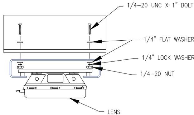
5. Bolt the radar to the mounted bracket using the supplied mounting hardware.
