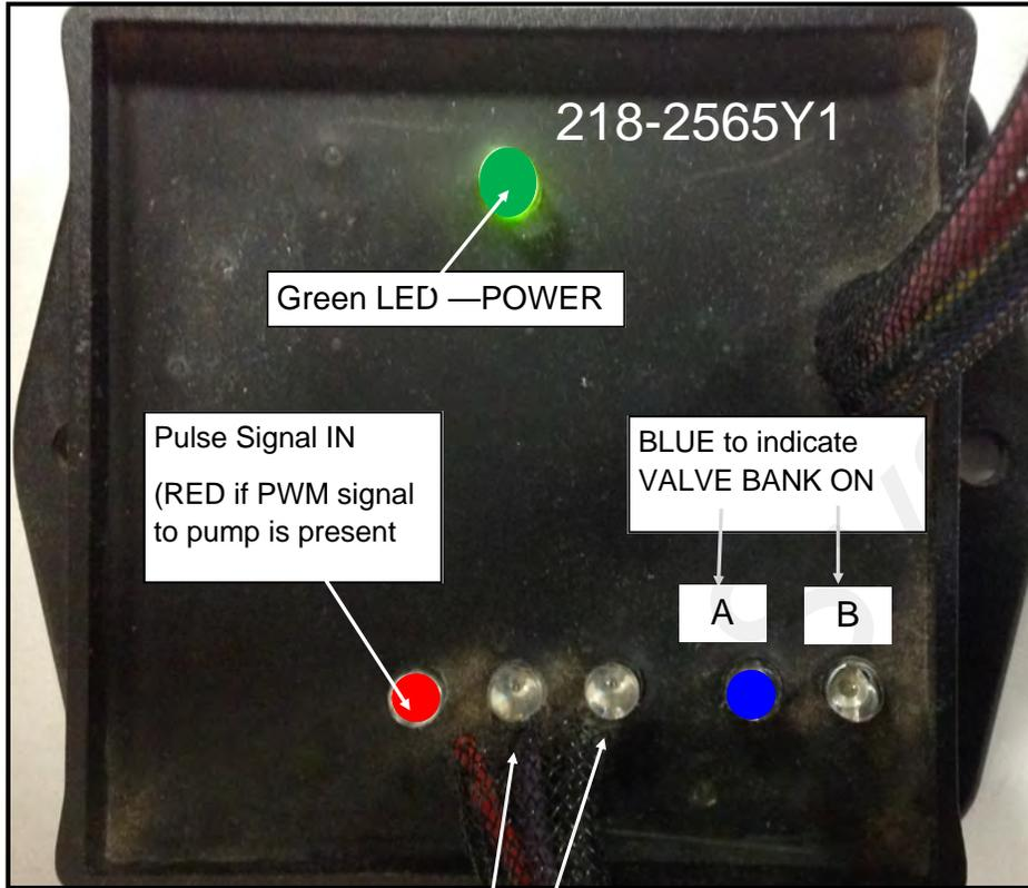
In **normal operation**, there should be a **Green** light, a **Red** light, and one or two **Blue** lights ON when the system is applying.
