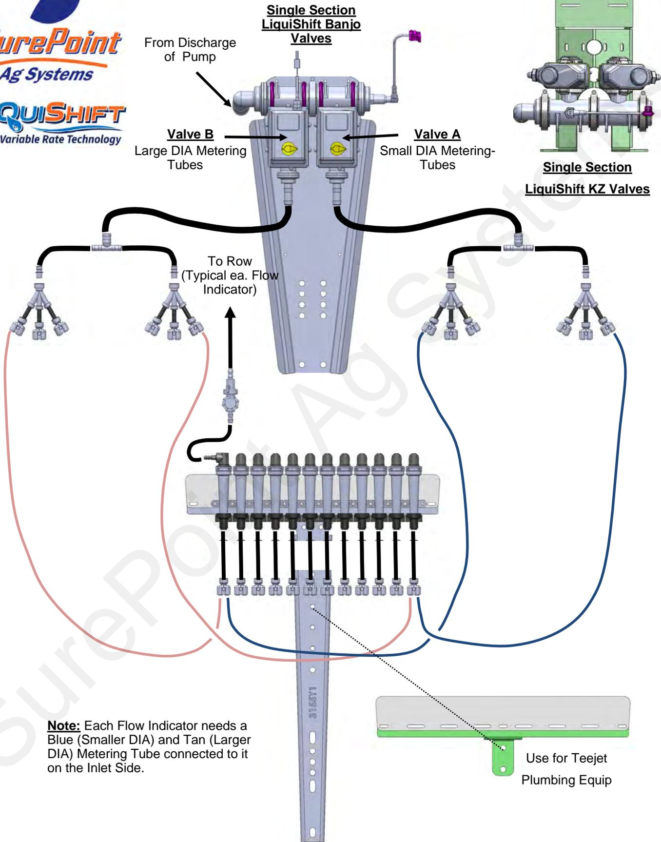
**Note:** Each Flow Indicator needs a Blue (Smaller DIA) and Tan (Larger DIA) Metering Tube connected to it on the Inlet Side.
