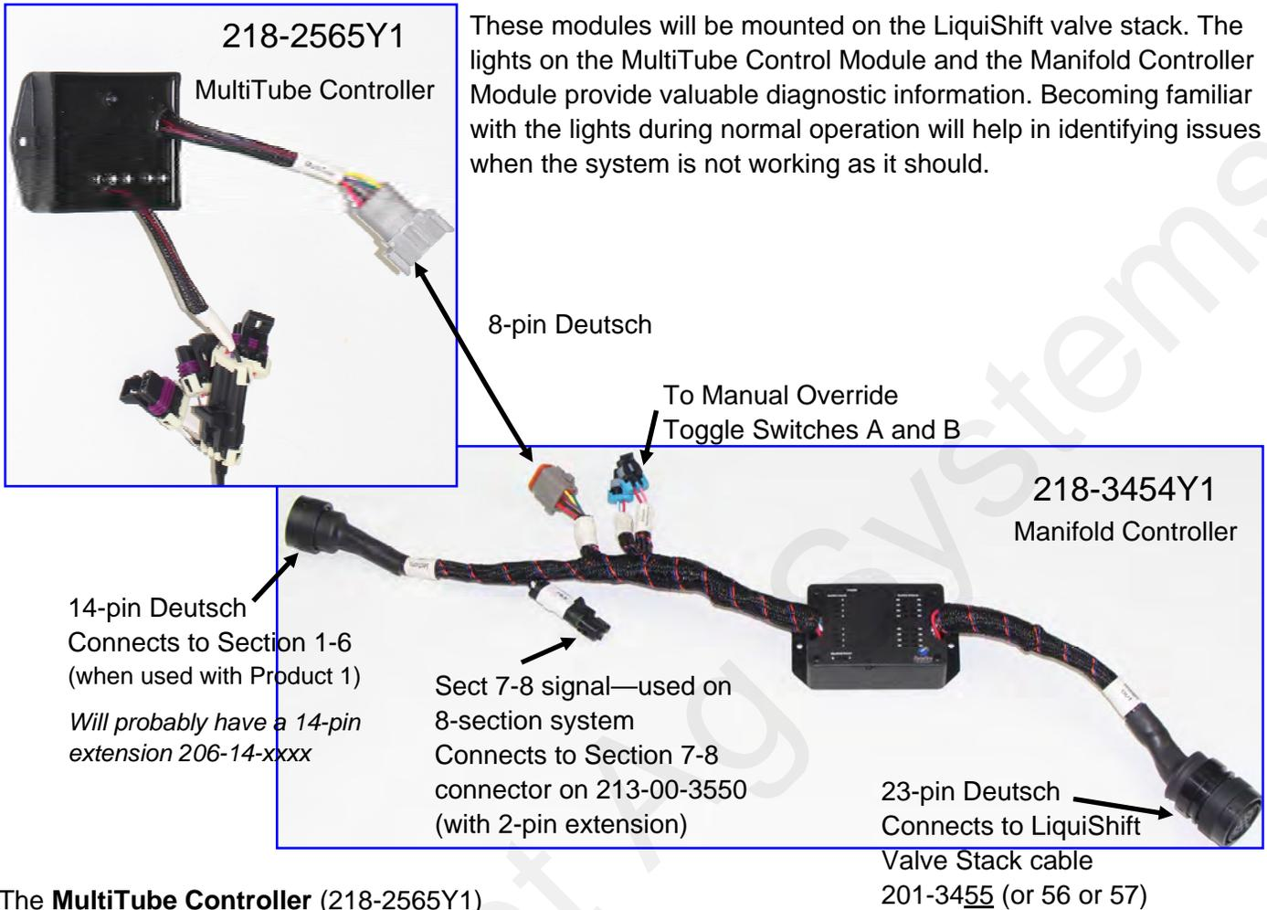
The **MultiTube Controller** (218-2565Y1) is mounted on the back of the LiquiShift tower, behind the **Section Manifold Control Module** (218-3454Y1).
