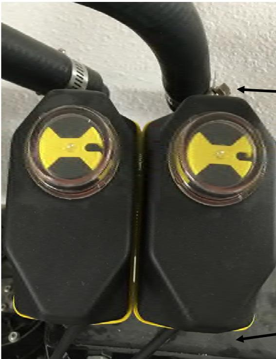
Product will flow through the bottom port when the valve is closed. (This can be used to return product to the tank when the system shuts off.) If the outlet to the row has been switched to the bottom port, the product will flow when the valve is closed, but will not flow when the valve is open.
