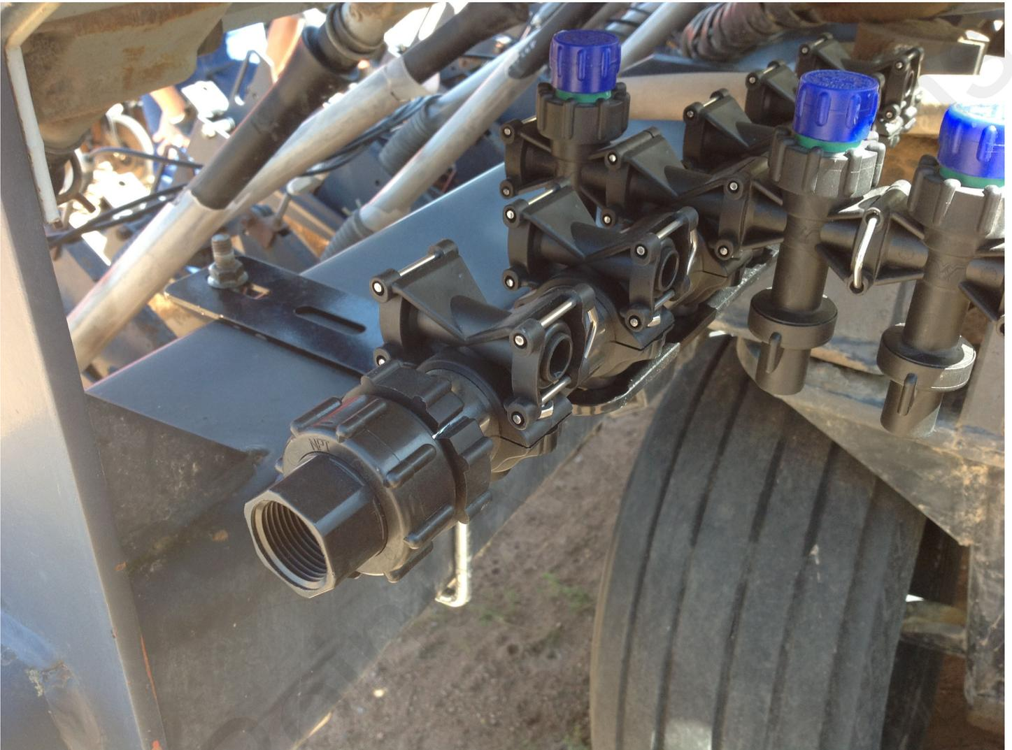
1. U-bolt manifold brackets to the 7"x7" bar under the box, roughly centered on the section.
