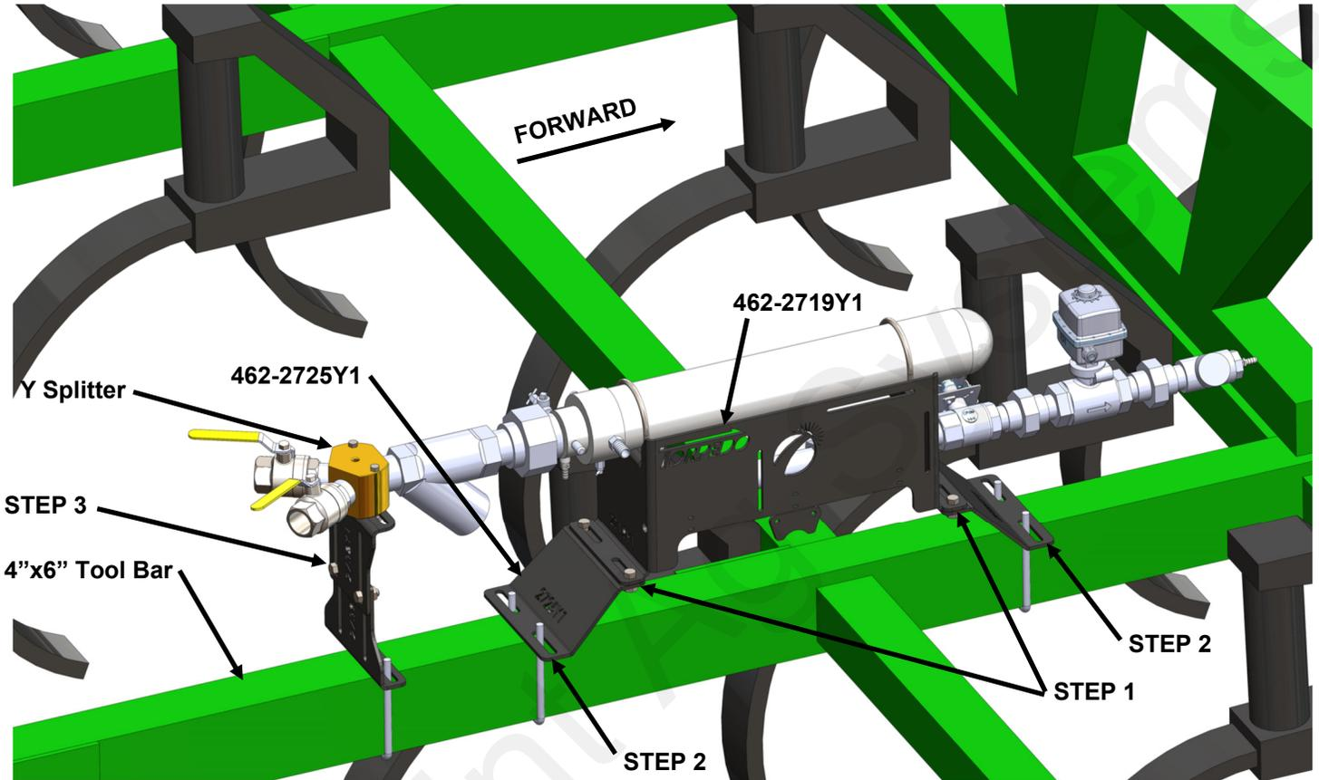
1. Bolt both "Z" Brackets (462-2725Y1) to the Torpedo Bracket (462-2719Y1) before mounting it to the 4"x6" Tool Bar using the provided 1/2" Bolts and Nuts.
