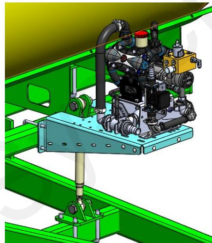
PumpRight pumps are fed with 1-1/2" hose from the valve in the plumbing kit below
