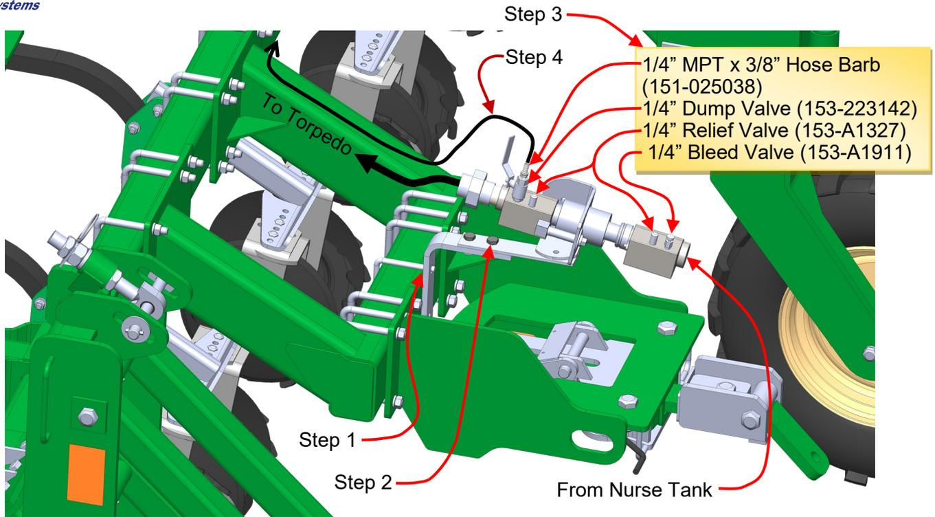
1. Mount the Break-Away Bracket (462-3277Y1-BK) to the Rear Hitch Bar/ Nurse Tank Hitch as shown, using the included 1/2"x6"x5" Square Bend U-bolt (380-1017). **Note: Recommended location of the Break-Away should be as far to the rear of the Implement as possible and as close to centered on the Implement as well. In doing so, this will optimize the functionality and safety of the Break-Away Coupler.**
