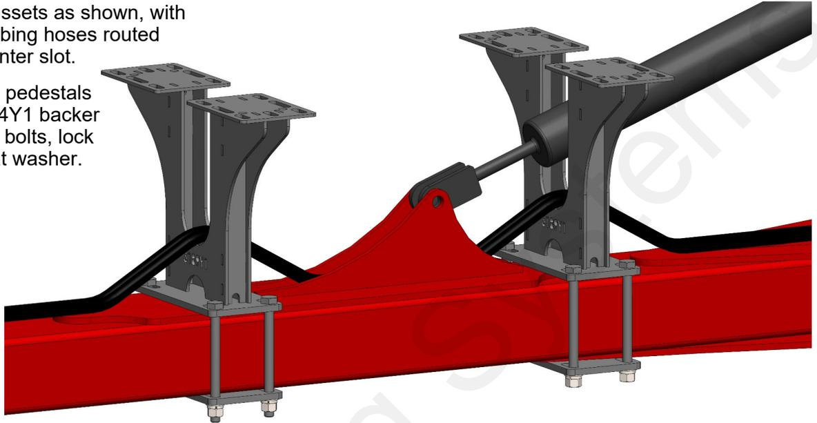
3. Bolt tank cradle to pedestal using four (4) 5/8" x 1-1/2" hex head bolts, flat washer and flange nuts for each pedestal.
