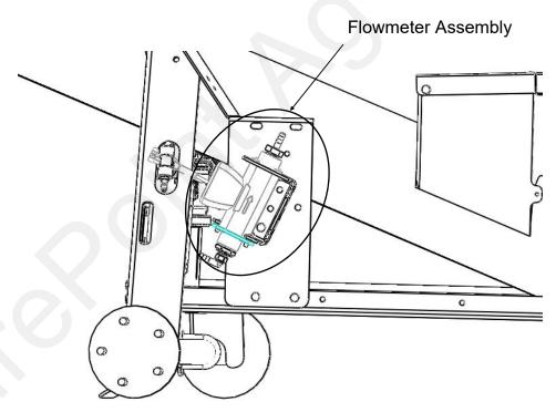
\*The calibration numbers in this publication are for flowmeters purchased after 10/15/2012. These flowmeters have a blue label with white text. Earlier flowmeters (with a white label with black text) have different calibration numbers.
