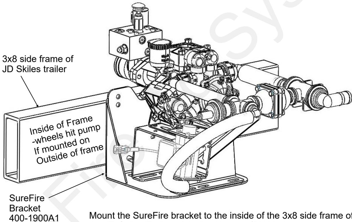
Mount the SureFire bracket to the inside of the 3x8 side frame of the JD Skiles Trailer. Attach with two 1/2" U-bolts.
