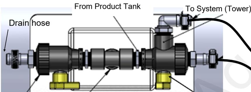
Drain Valve to drain tank—1/4 turn valve to open or close drain
