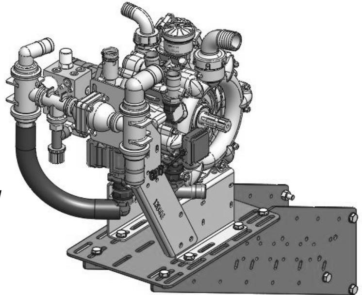
1. Attach the top plate (400-1314A1) to the side plates using four (4) 1/2" x 1-1/2" Hex Head Bolts, flat washers, and flange nuts as shown below. Tighten finger tight.
