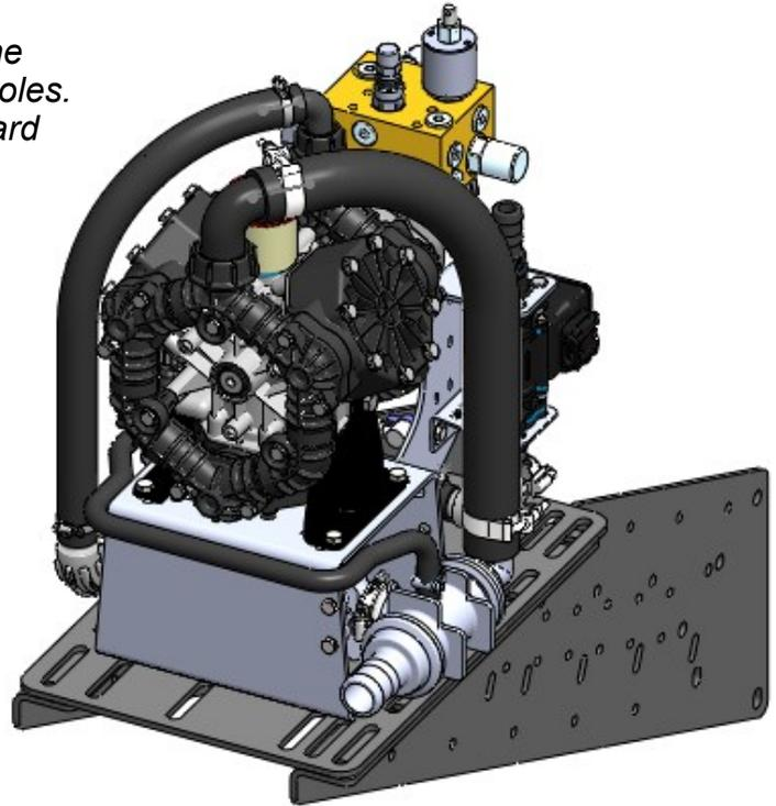
1. Attach the top plate (400-1314A1) to the side plates using four (4) 1/2" x 1-1/2" Hex Head Bolts, flat washers, and flange nuts as shown below. Tighten finger tight.
