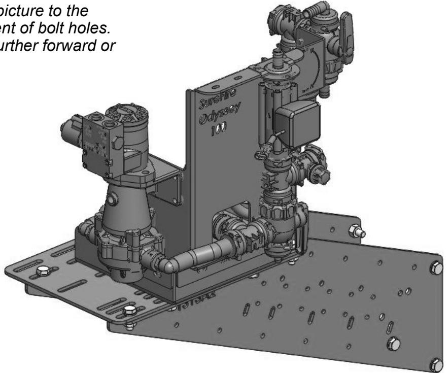
1. Attach the top plate (400-1314A1) to the side plates using four (4) 1/2" x 1-1/2" Hex Head Bolts, flat washers, and flange nuts in the four corners. Tighten finger tight.
