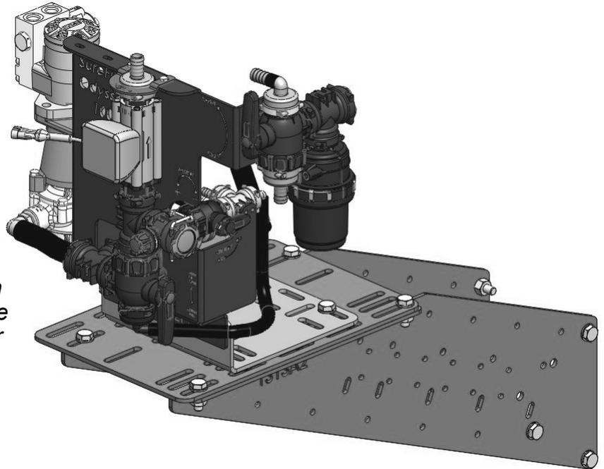
1. Attach the top plate (400-1314A1) to the side plates using four (4) 1/2" x 1-1/2" Hex Head Bolts, flat washers, and flange nuts in the four corners. Tighten finger tight.
