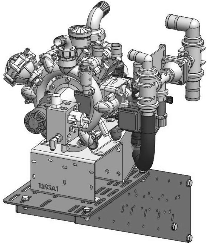
1. Attach the top plate (400-1314A1) to the side plates using four (4) 1/2" x 1-1/2" Hex Head Bolts, flat washers, and flange nuts as shown below. Tighten finger tight.
