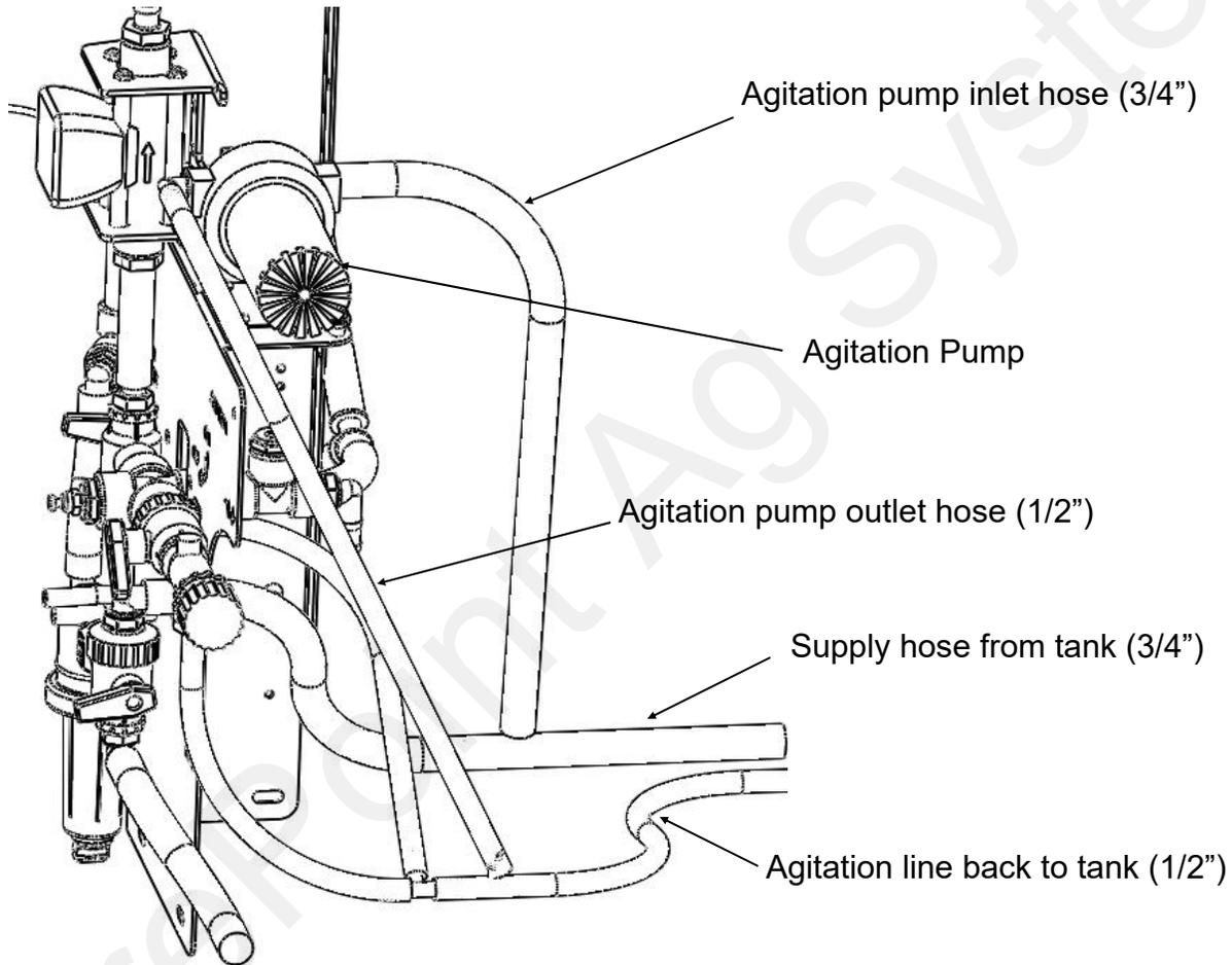
This kit provides an electric pump that provides dedicated agitation flow for the Tower 200. This would work on any tank mounting, but is designed specifically to agitate the Accelerator tank with jet agitator in the bottom of tank. To install:
