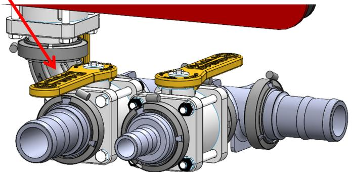
3. Assemble strainer fittings and install hose as shown.
