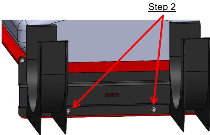
2. Install the bottom using two (2) 5/8" x 1-1/2" hex head bolts, washers, and nylock nuts
