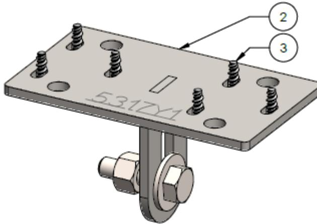
1. Attach Zip Valves to the mounting bracket using the provided Thread Forming Screws. *Do not overtighten.*
