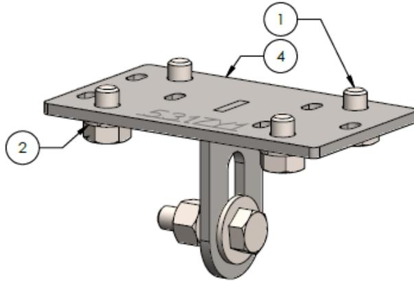
1. Attach Sentinel Row Control Valves to the mounting bracket using the provided hardware.
