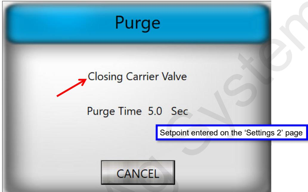
After the valves are closed, the purge valve will open. While the purge valve is open the indicator light on the top of the QuickDraw will be on (not flashing) and the following screen will be visible:
