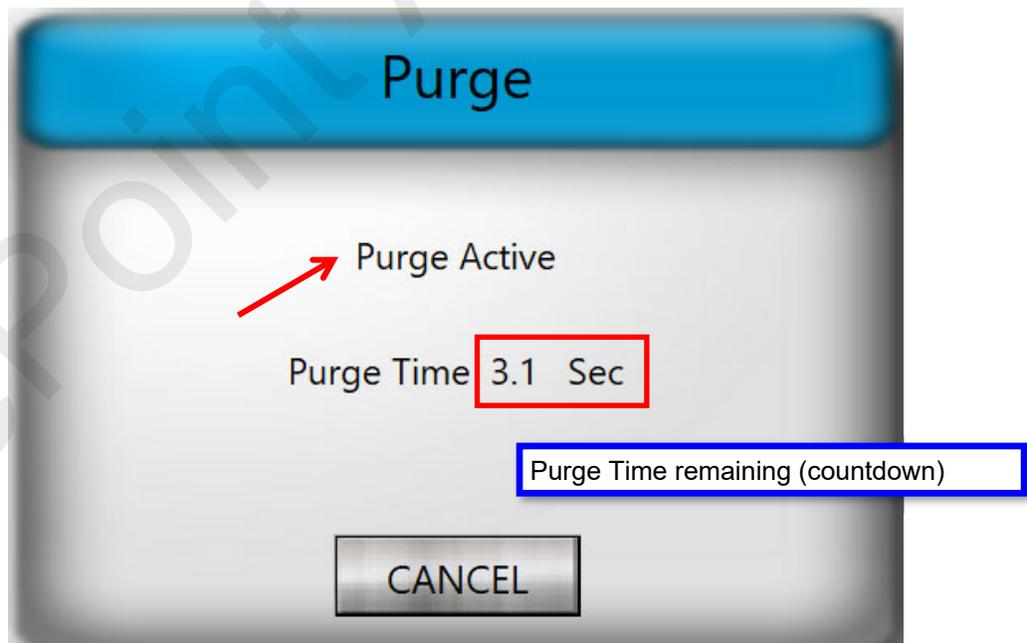
The Purge Time will count down, indicating how long the purge valve will remain open. When the purge cycle is complete, the indicator light on the top of the QuickDraw will turn off.
