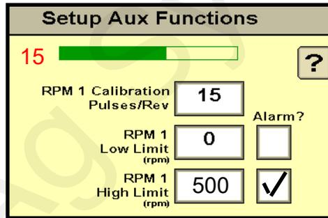
If pump suddenly needs more RPM to reach output, check for restrictions on the inlet side (strainer, etc).
