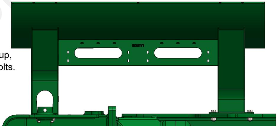
4. Finally, install the tank in the saddles and fasten the tank strap mounting brackets, and tank straps. Check for clearance from seed boxes when folding and when the drill is raised and lowered. Note: Tighten straps again once the tank has been filled.
