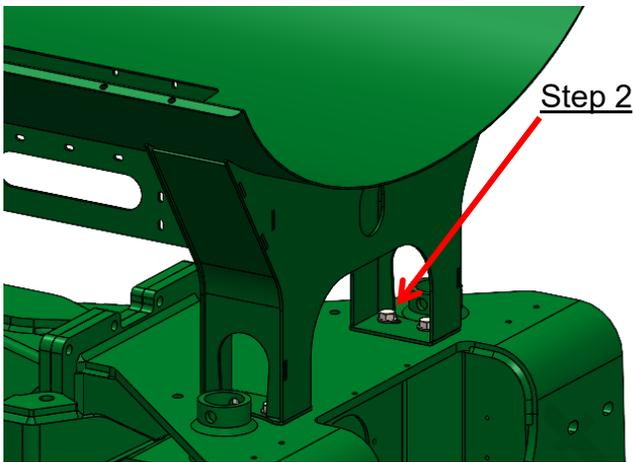
2. Loosely mount the back of 450-5000Y1 to the bolt plate on the hitch using four (4) 3/4" x 2-1/2" hex head bolts, washers, and flange nuts.
