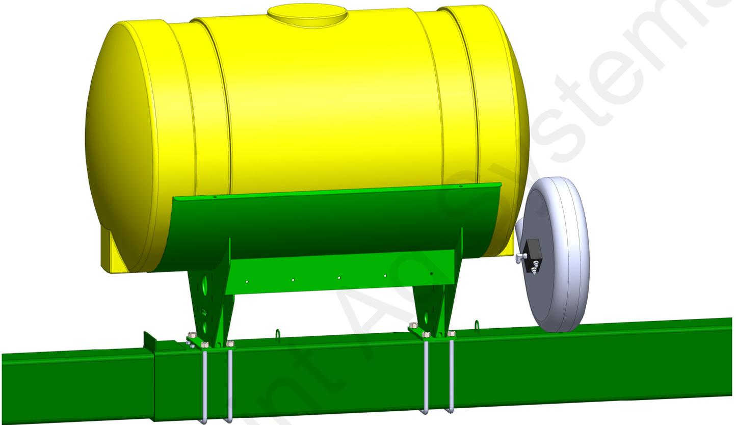
1. Loosely attach 400-2088Y1 tank cradle on John Deere 8"x12" hitch using four (4) 3/4" x 8" x 13-1/2" square bend u-bolts. Note: See next page for dimensions and further mounting instructions.
