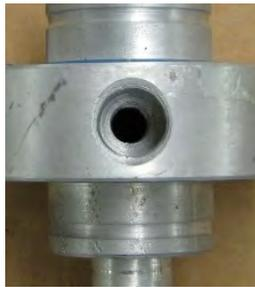
Threaded orifice not installed
