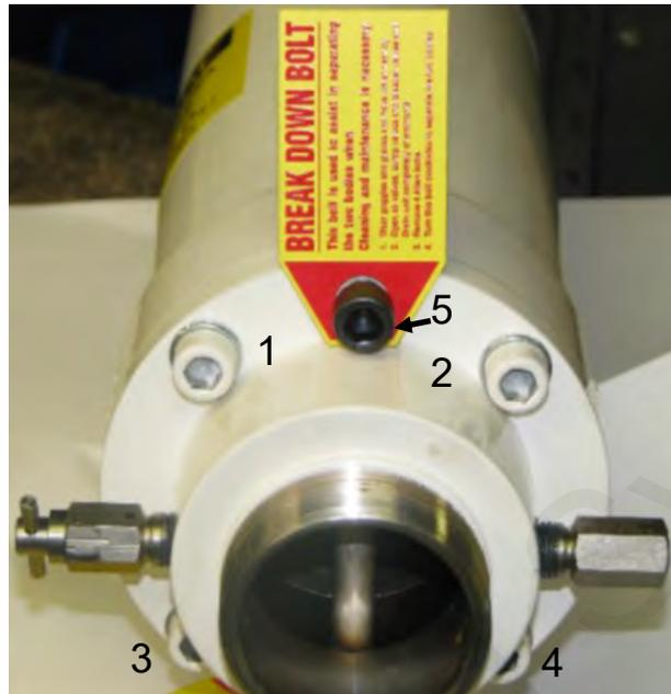
2. Replace both inner o-ring dump seals and body o-ring seal. Repair kit part number 153-01-A-SF-RK.
