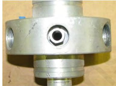
Threaded orifice installed
