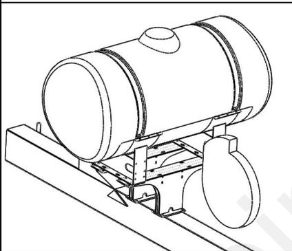
This is the only tank option that works with the CaseIH Central Fill Seed system. The tank sits in front of the central fill seed and behind the vacuum fan mounted on the left wing. This tank WILL NOT work on 12 row planters with markers. It will fit 16 row planters with markers
