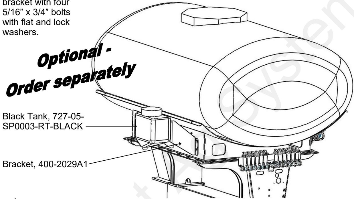
Bracket mounts to 2 slots on each side of opening in tank cradle. Rinse tank can mount on either side of the tank.
