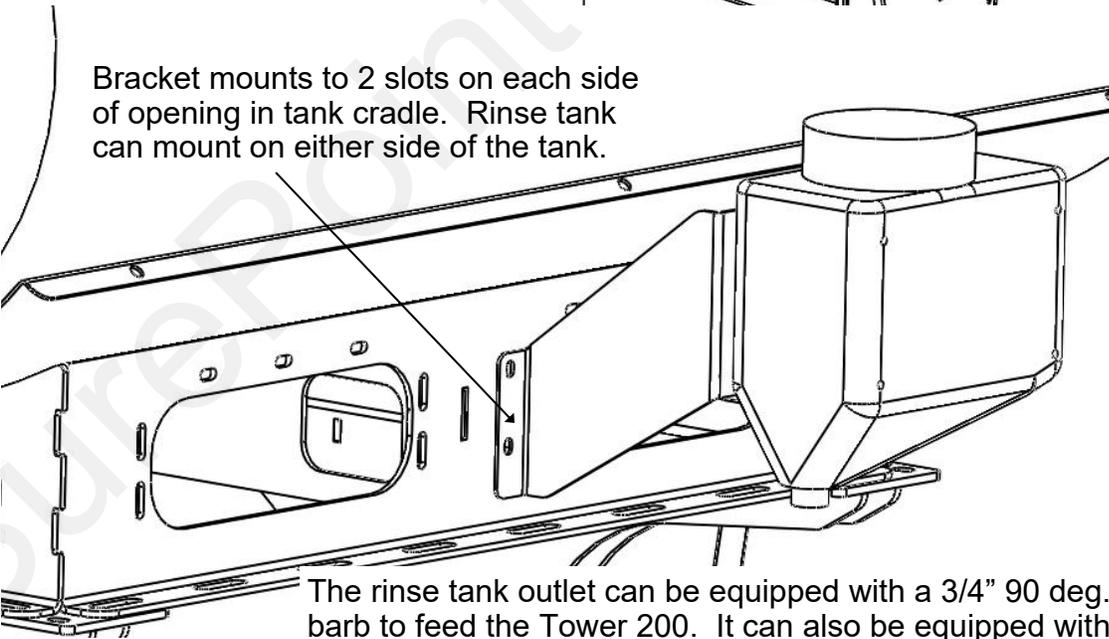
The rinse tank outlet can be equipped with a 3/4" 90 deg. hose barb to feed the Tower 200. It can also be equipped with a valve for hand wash. A tee can be used to feed both the tower 200 and hand wash valve.
