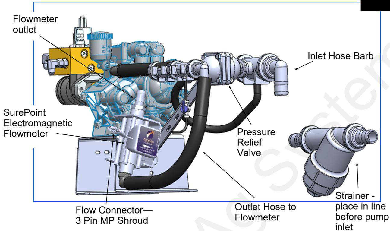
**Inlet:** The D70 and D115 PumpRight is shipped with a 1 1/2" inlet hose barb. Attach this to the hose from your supply tank and strainer. A 1 1/2" 90 degree hose barb is included and can be substituted.
