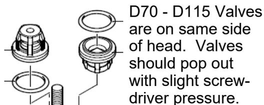
D70 - D115 Valves are on same side of head. Valves should pop out with slight screwdriver pressure.
