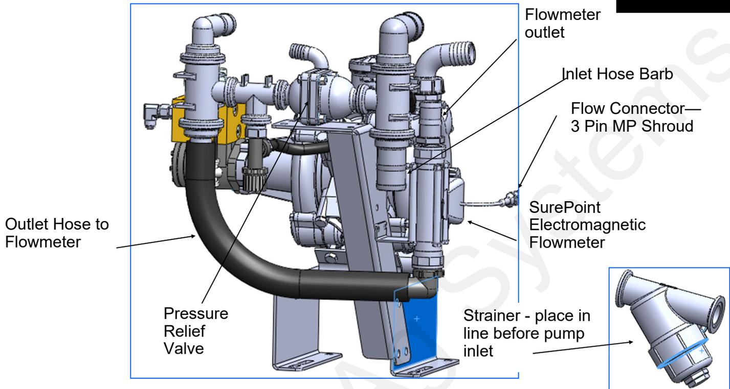
**Inlet:** The D160 and D250 PumpRight is shipped with a 2" inlet hose barb. Attach this to the hose from your supply tank and strainer. A 2" 90 degree hose barb is included and can be substituted.
